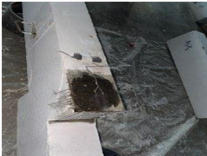
Figure 3.27 Strain gauges attached to the beam.
