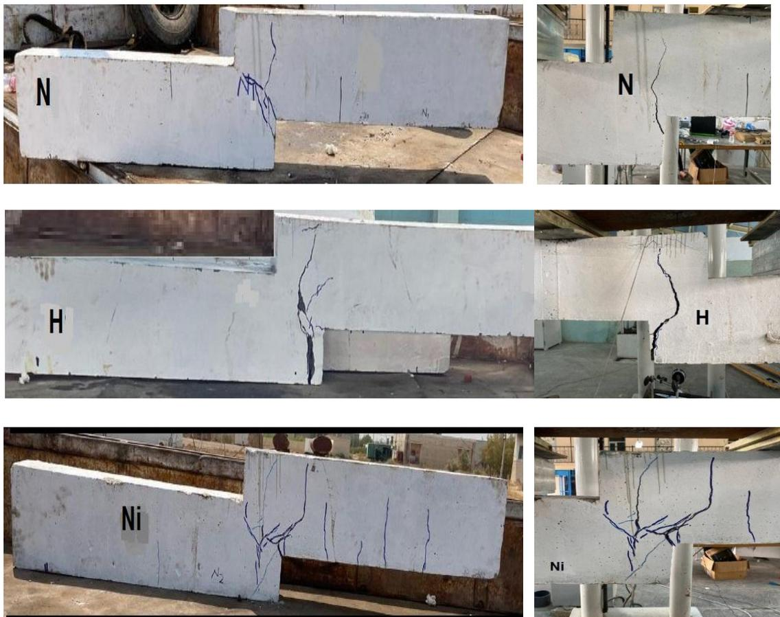
Figure 4.9 Cracks pattern for beams.
