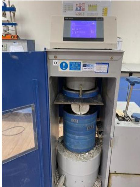
Figure 3.23 Split tensile strength test.
