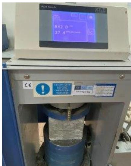
Figure 3.22 Compressive strength test.
