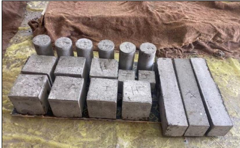
Figure 3.21 Specimens of hard concrete tests (cubes, cylinders and prism).
