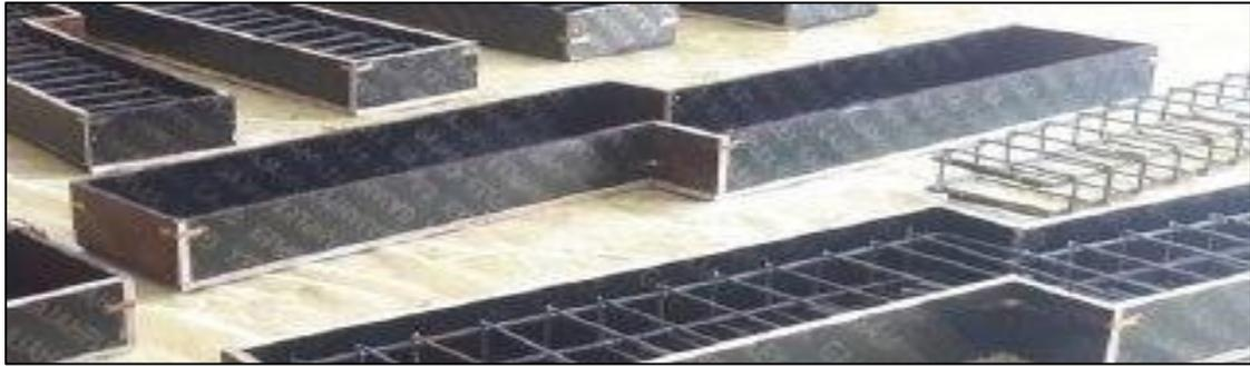
Figure 3.18 Beam molds.
