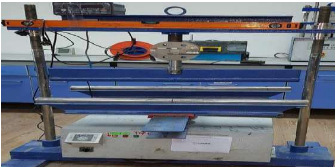
Figure 4.4 Modulus of rupture test device.
