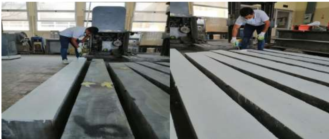
Figure 3.30 Paint the beams.
