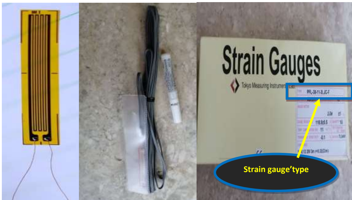
Figure 3.25 The strain gauge types used in this research.
