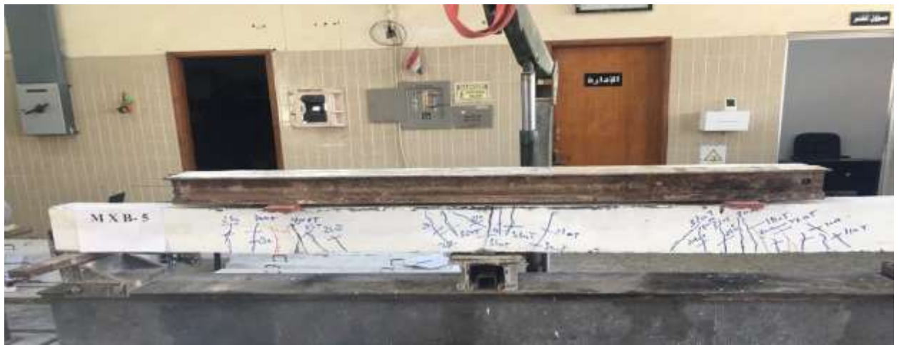
Figure 4.9 Crack pattern of MXB-5 (1.5% S.F).
