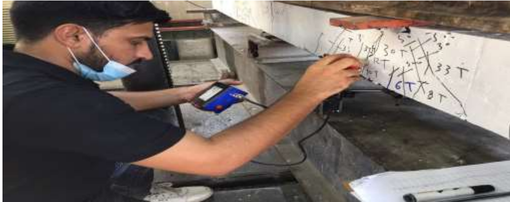
Figure 3.28 Record width of cracks.
