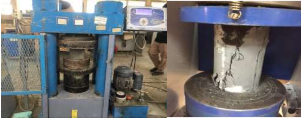
Figure 3.17 Compressive Strength Test.
