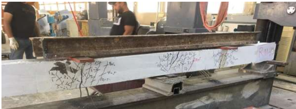
Figure 4.15 Crack pattern of RM-B (solid).
