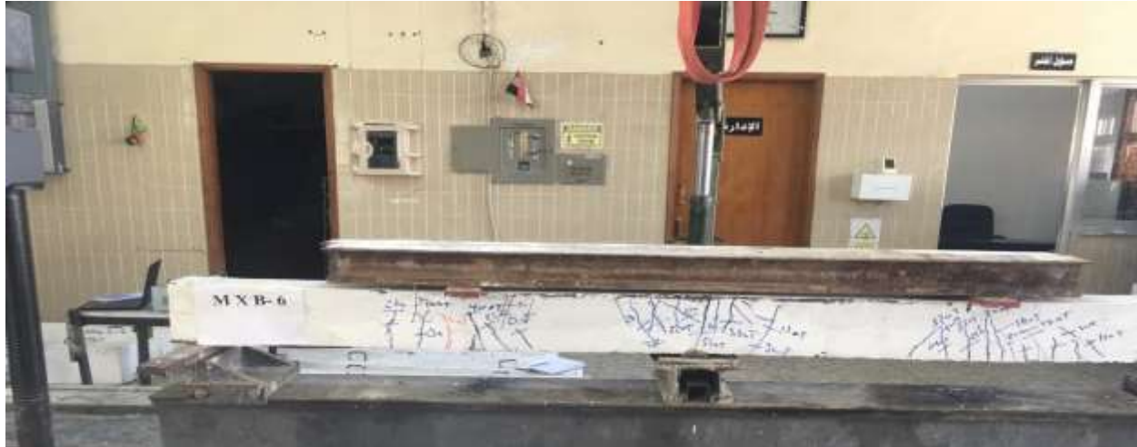
Figure 4.10 Crack pattern of MXB-6 (2% S.F).
