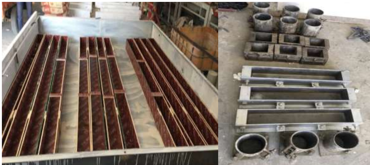
Figure 3.9 Wood mold and steel molds for cubes, cylinder and prism
