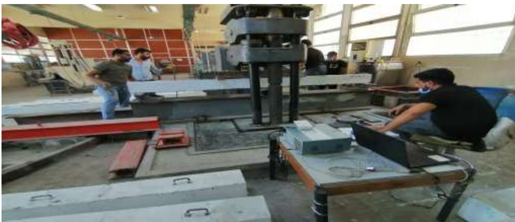
Figure 3.27 Beams under test.
