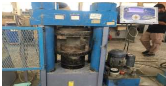
Figure 4.3 Cube Compressive Test.
