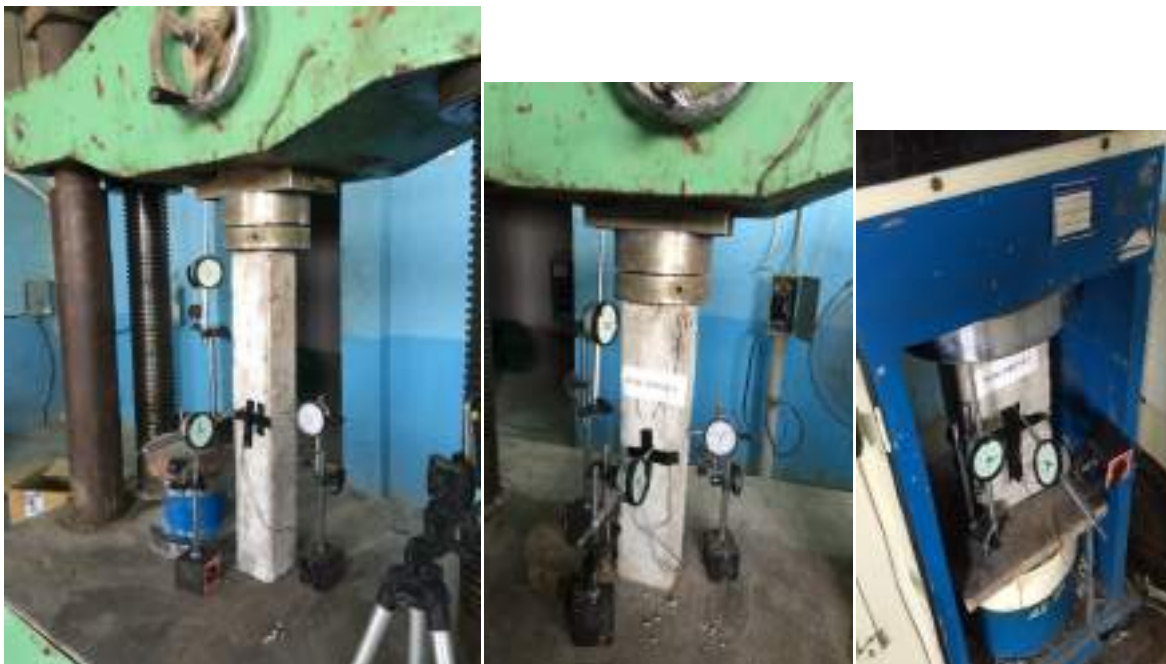
Figure (3- 39) Install concrete column specimens inside the machine
