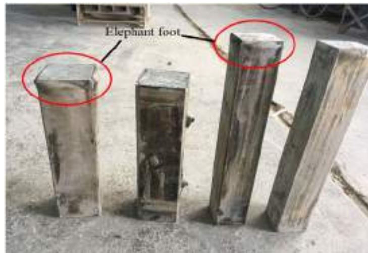
a) Elephant foot failure
