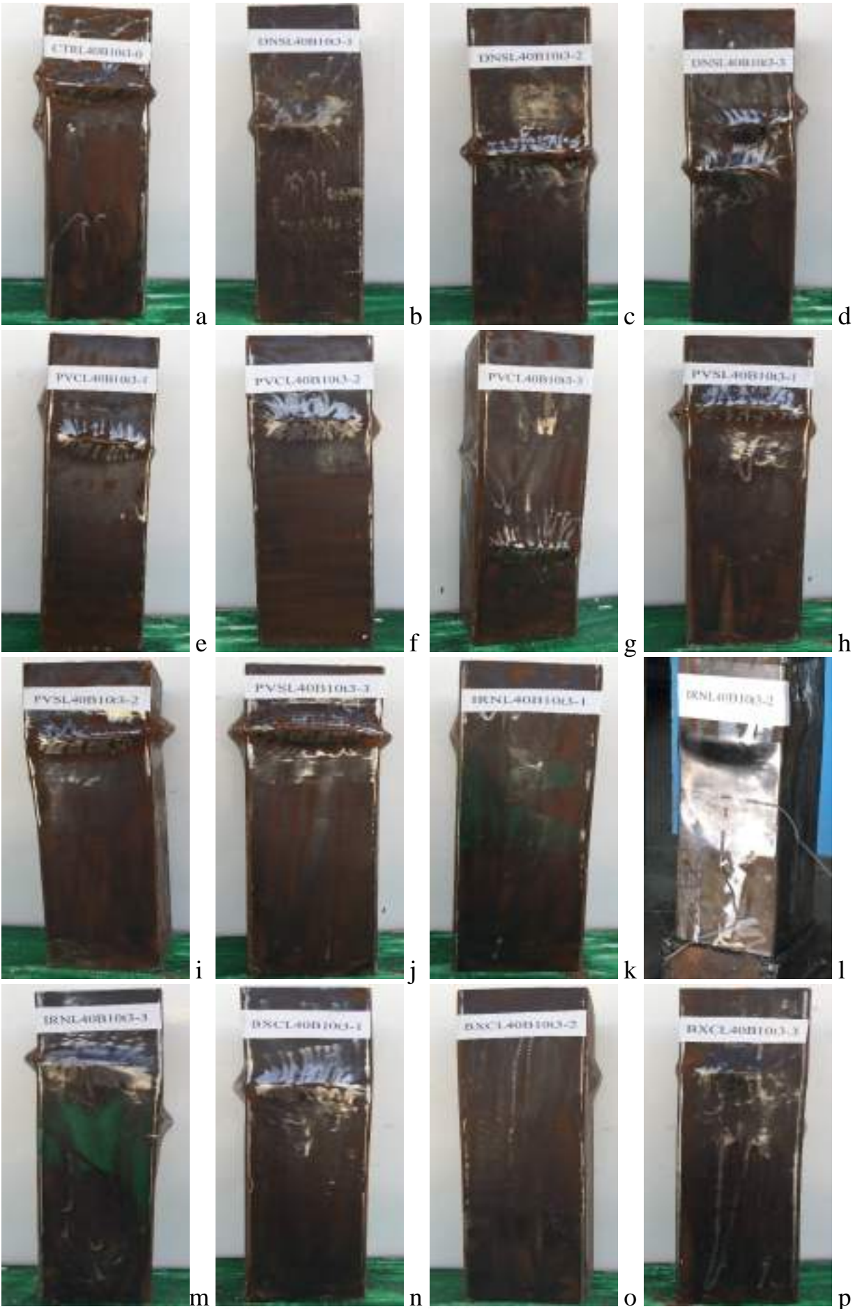
Figure (4- 81) Mode of failure of (CFST) short column specimens
