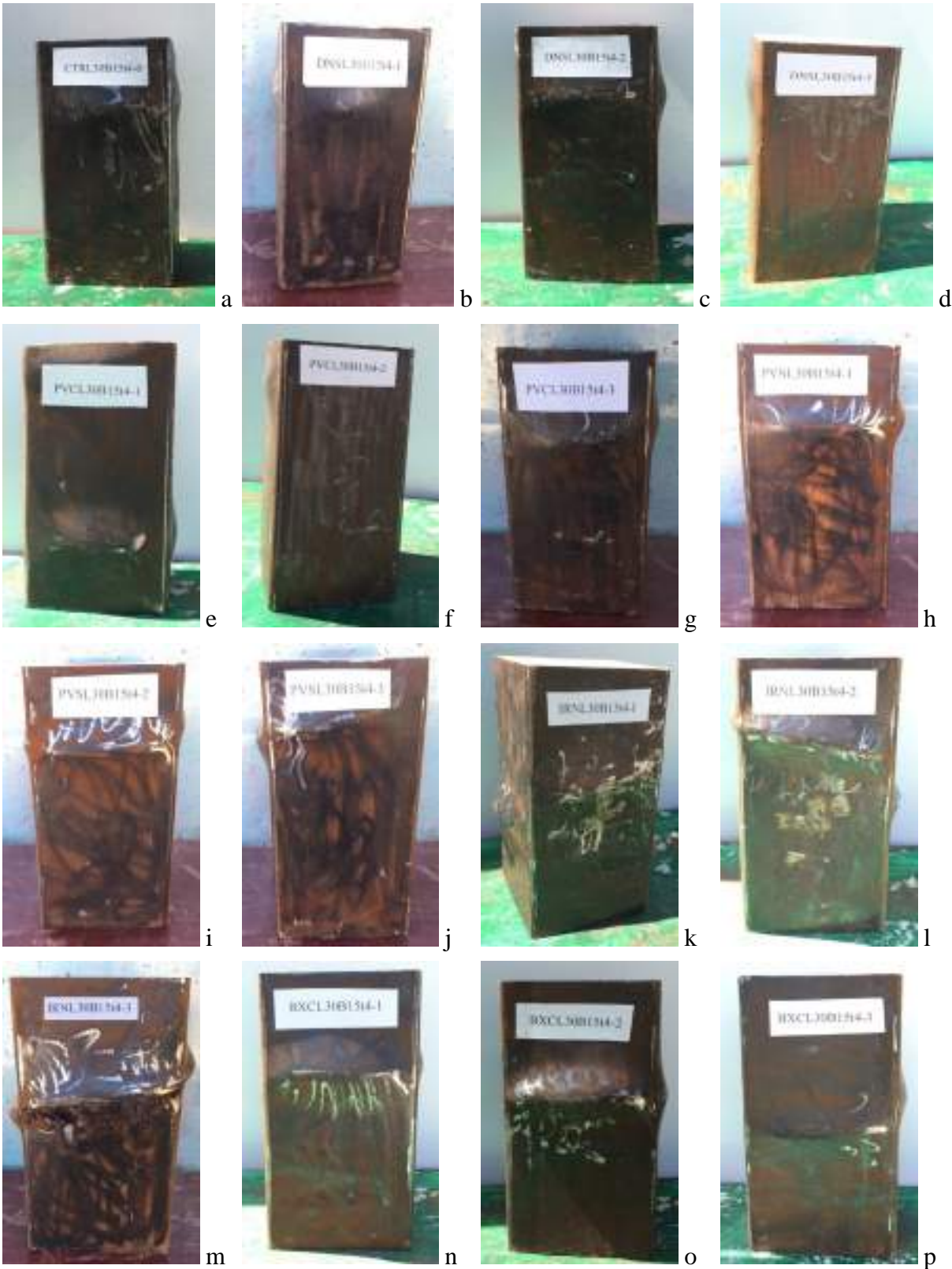
Figure (4- 52) Mode of failure of (CFST) stub column specimens
