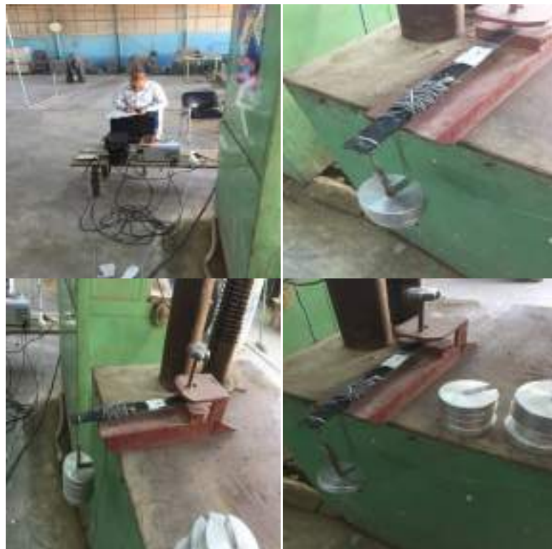
Figure (3- 29) Tool of calibration of strain gauges
