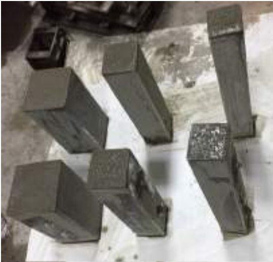
a) Casting of (CFST) specimens
