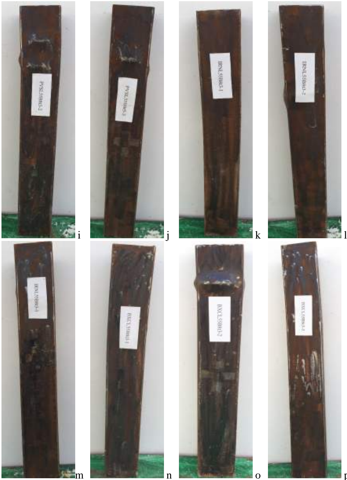
Figure (4- 110) Mode of failure of (CFST) long column specimens
