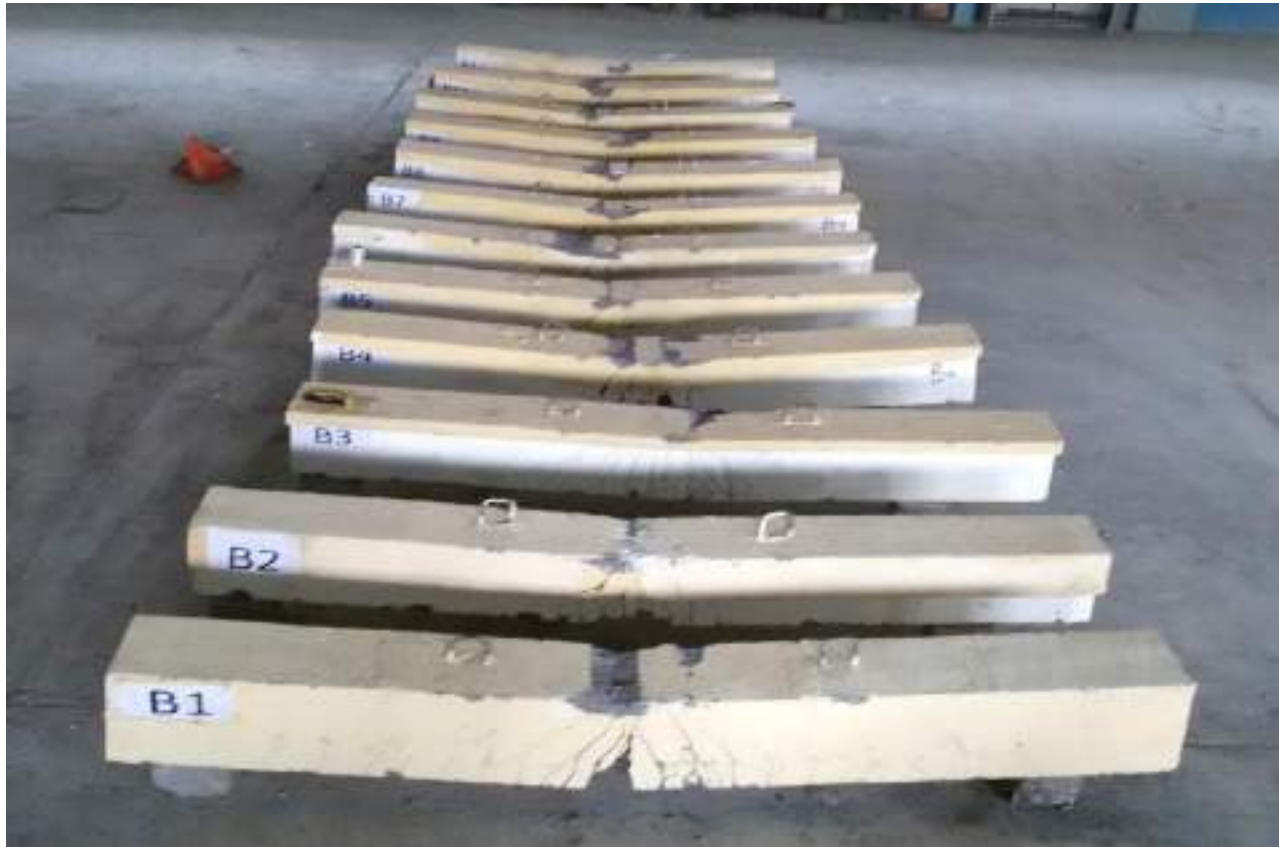
Figure (4-15) Tested beam sets
