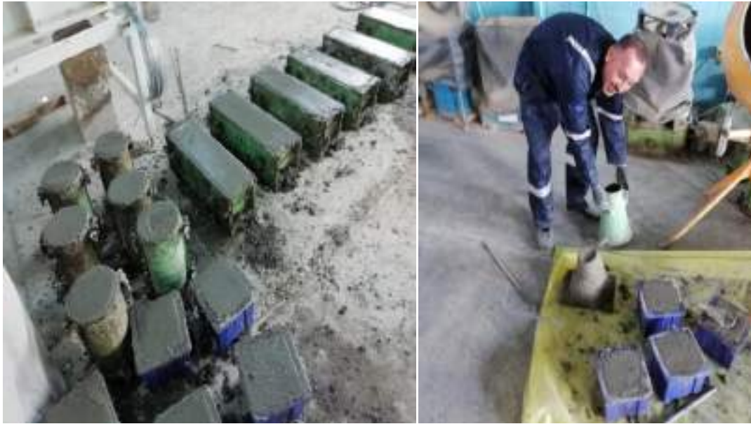
Figure ( 3-8 ) Casting Processes Samples and slump test
