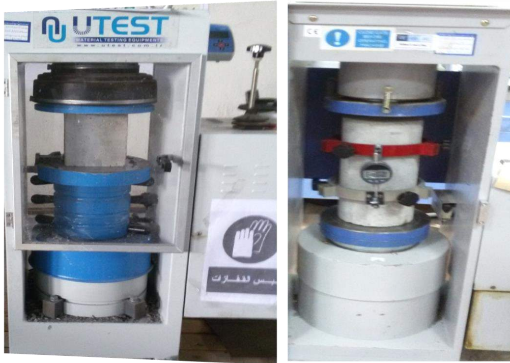
Figure ( 3-4 ) Compressive strength test
