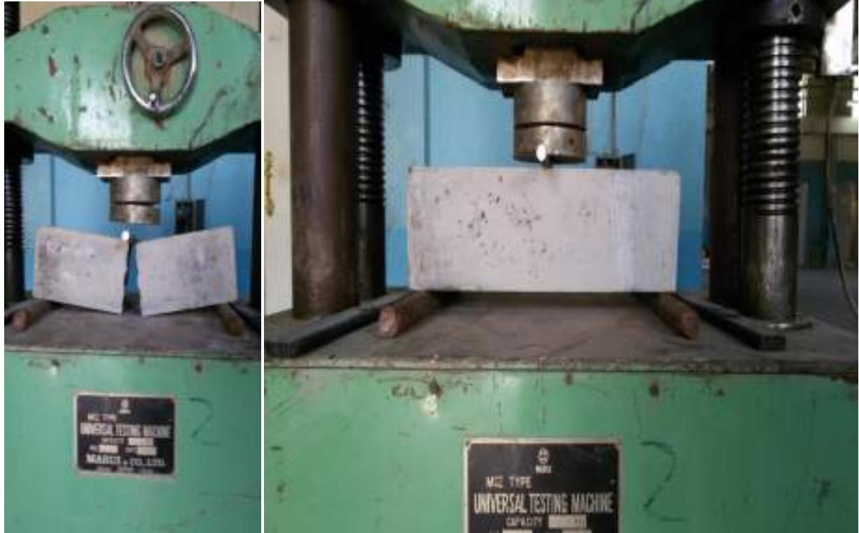
Figure ( 3-6 ) Flexural strength test
