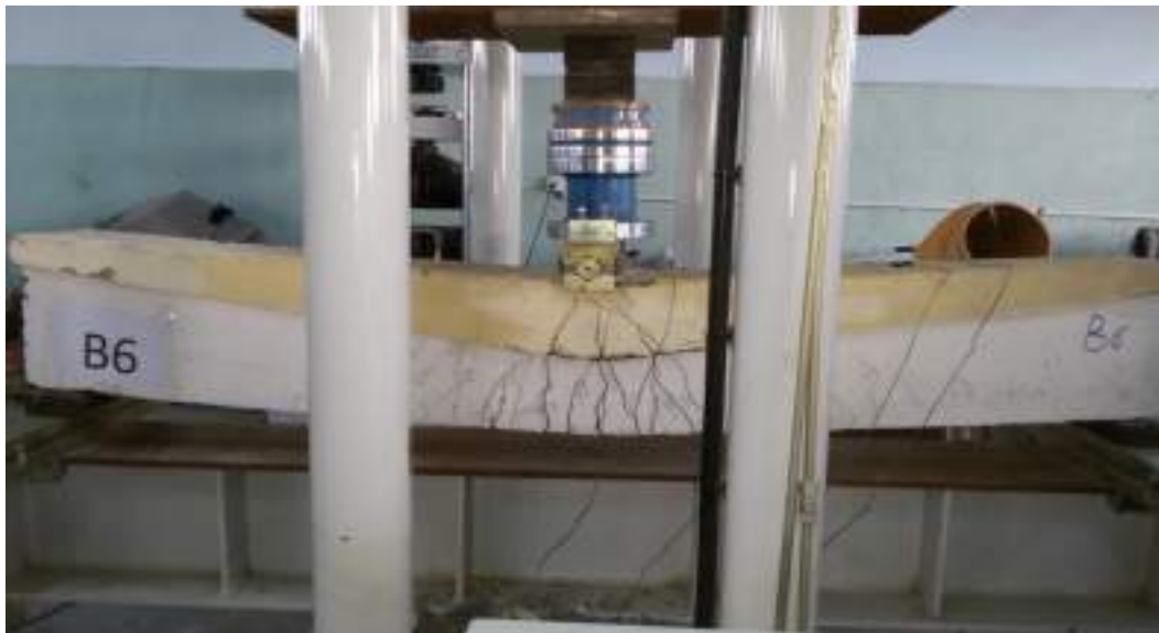
Figure (4-14) Typical failed specimens under test setting
