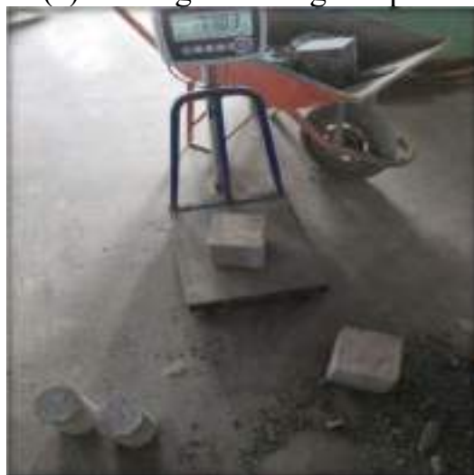
(c) Weighting of concrete samples
