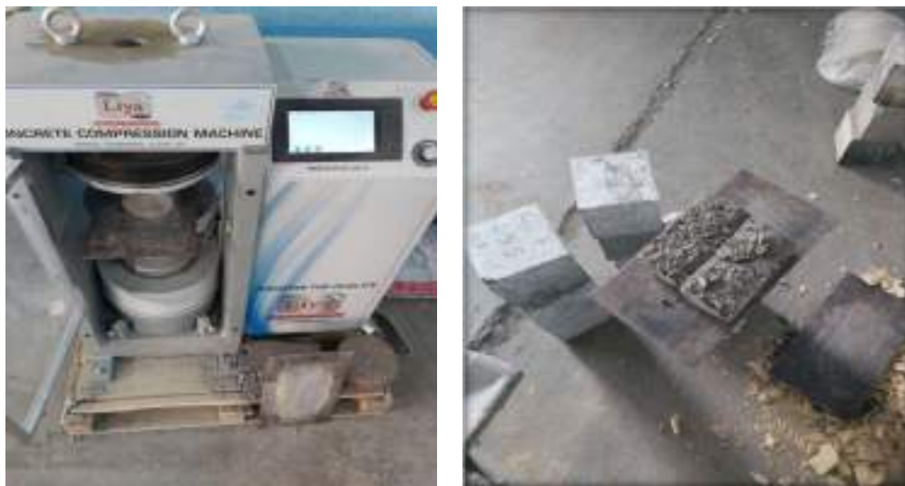
Figure 3. 22 Split tensile test machine
