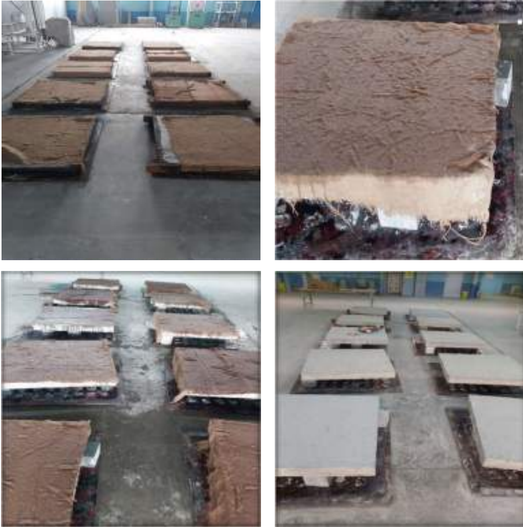
Figure 3. 18 Curing of waffle slab specimens.
