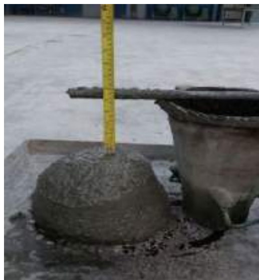
Figure 3. 20 Workability tests, Slump.
