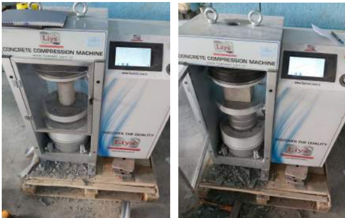
Figure 3. 21 Compression strength test.
