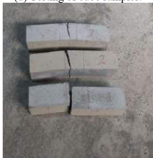
(f) Concrete prisms after testing.
