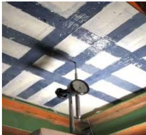
Figure 3. 29 Dial Gauge Deflection.
