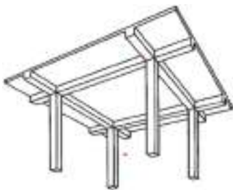
(1) classical slab with cross beams
