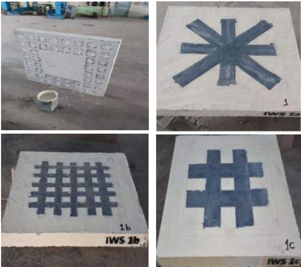
Figure 3. 26 Specimens' paintings, CFRP bonding, and marking.
