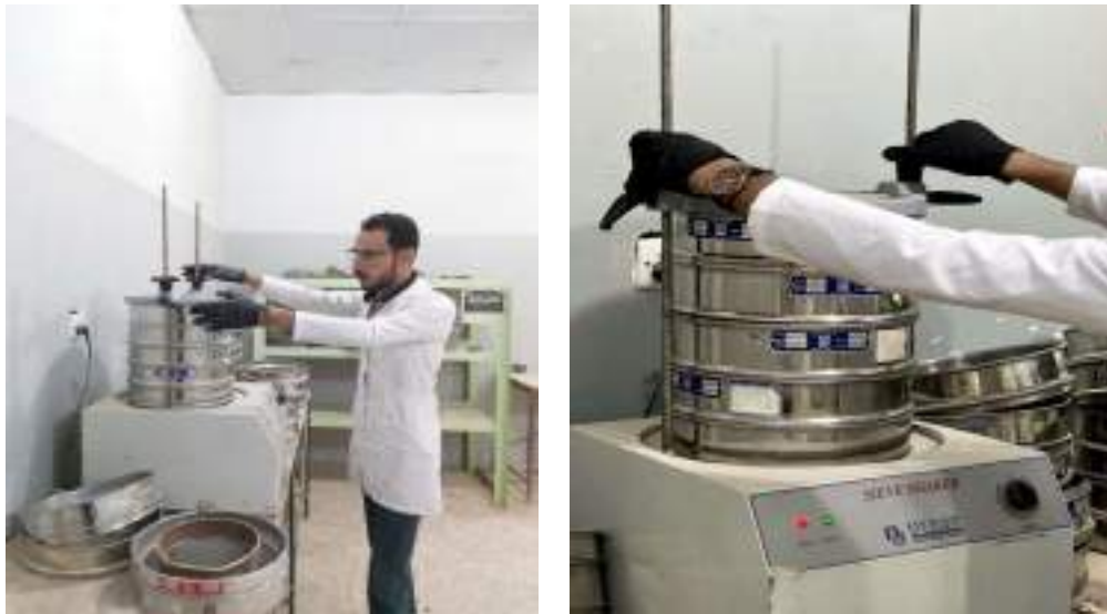
Figure 3. 9 Coarse aggregates (air dried) sieve analysis.
