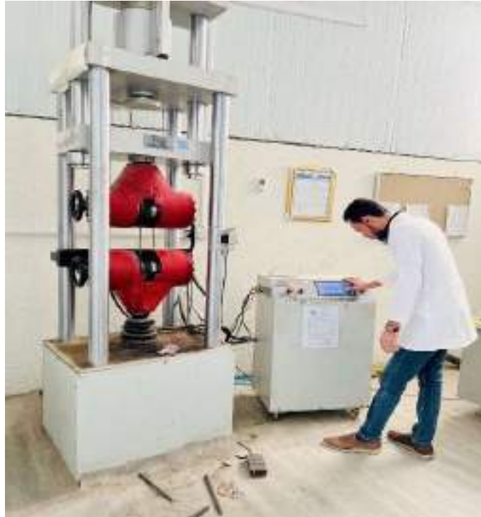
Figure 3. 12 Machine Used for Steel Bars.
