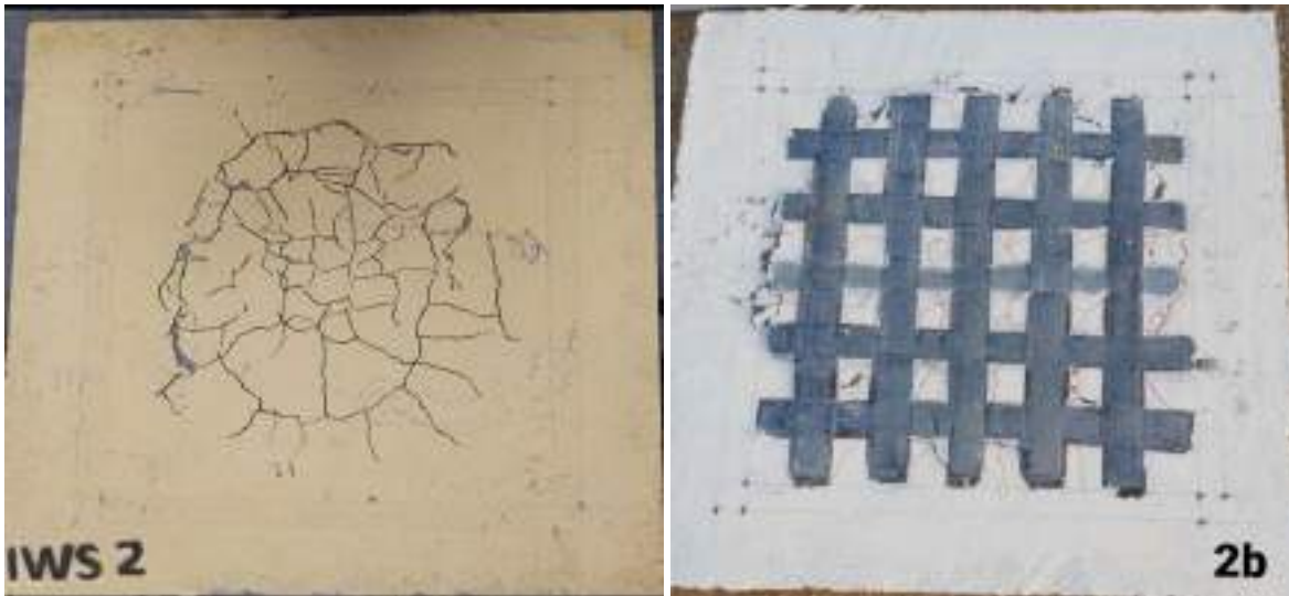
Figure 4. 20 Failure crack pattern
