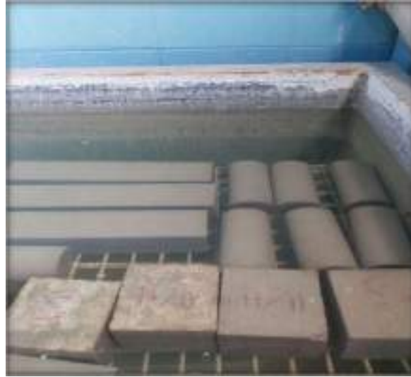
Figure 3. 19 Curing of concrete samples.
