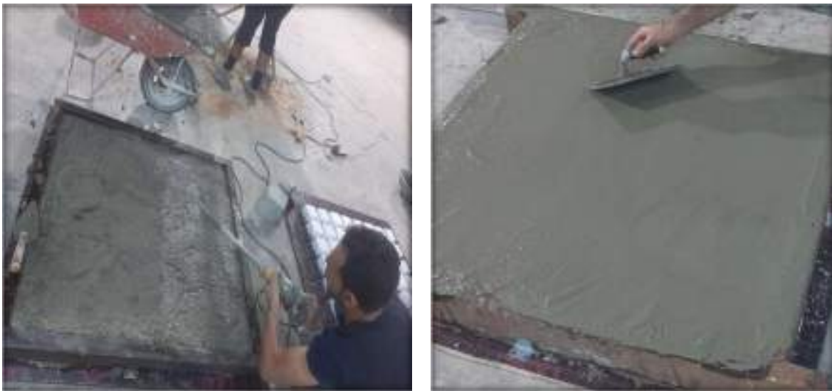
Figure 3. 17 Specimens casting, vibrating, and finishing.
