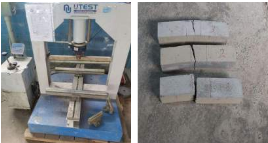
Figure 3. 23 Flexural testing machines.
