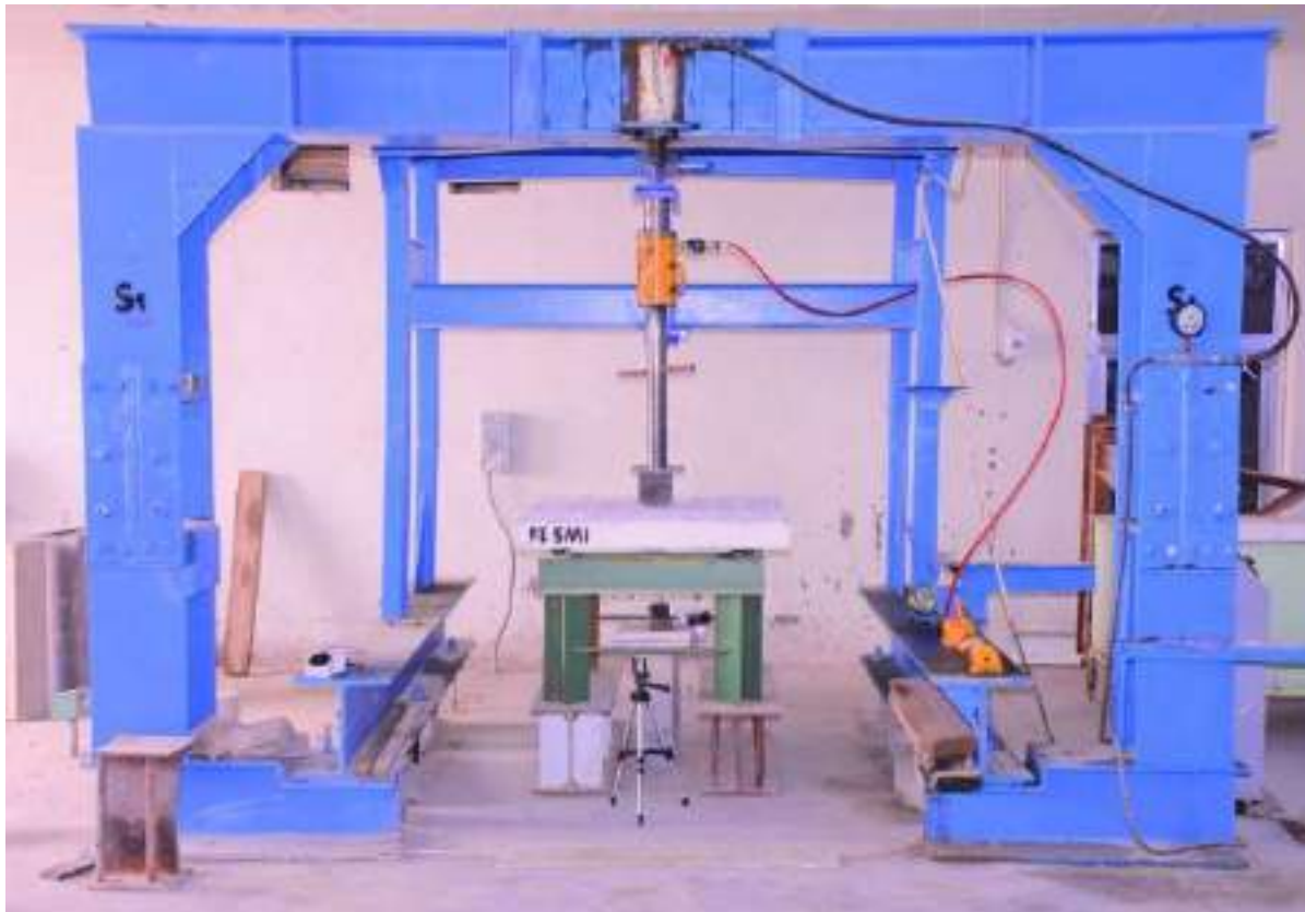
Figure 3. 27 Testing Framed machine and waffle slab specimen.
