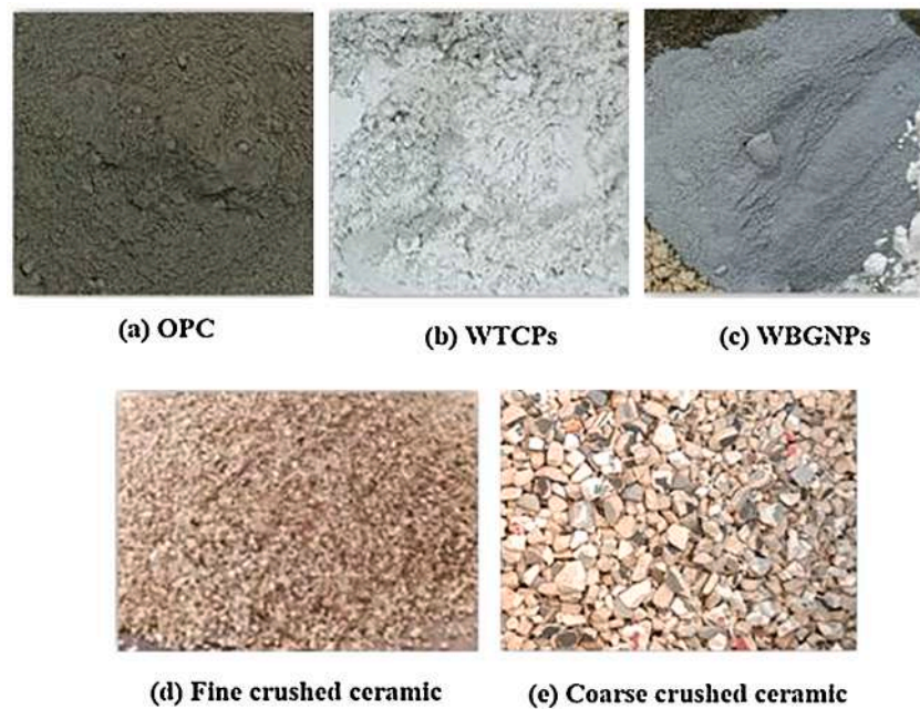
Fig. 1. Raw materials used in preparing the modified concrete specimens: (a) OPC, (b) WTCs, (c) WBGs, (d) fine crushed ceramic ( \leq 4.75 mm), and (e) coarse crushed ceramic ( \leq 10 mm).
