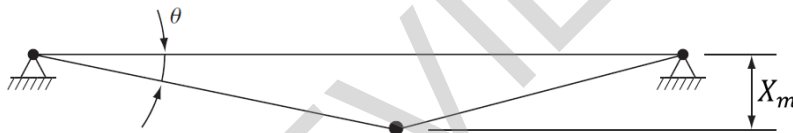
Figure 2.12. Member (beam, slab, or panel) support rotations (DoD, 2008).
