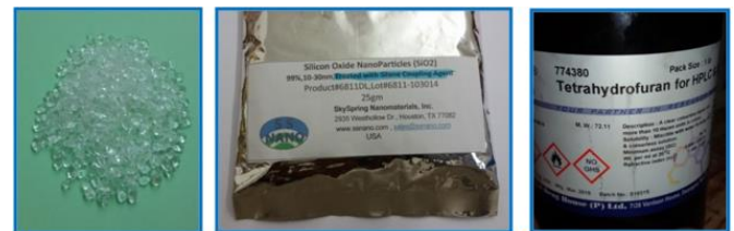
Fig. 11 (a) PMMA granules, (b) silicon oxide nanoparticles ( \text{SiO}_2 ) and (c) tetrahydrofuran solvent.
