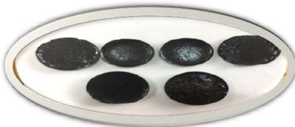
Figure 5. Image of cured PFA used in chemical resistance study before immersion in chemical solution.
