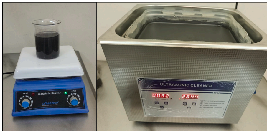
Fig. 3. Ultrasonic cleaner and magnetic stirrer of GnP/water.
