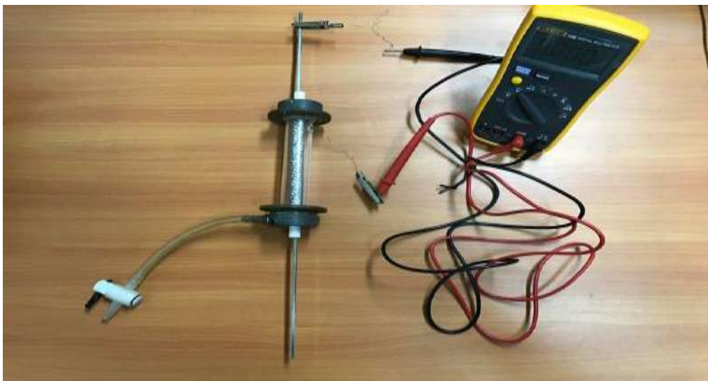
Figure 3.13 Represents the Basic Cell which Used in the Measurement of Zeta Potential, Consist of the Ceramic Membrane was Mounted in Transparent uPVC Module House, Outside Electrode and Inside Electrode were Connected to Nigh Impedance Milli-Voltmeter.
