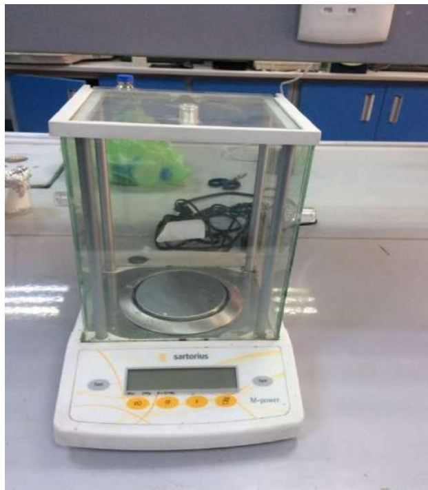
Figure B.1.10 Digital Balance (AZ214 supplied by Sartorius Weighing Technology GmbH, Germany)
