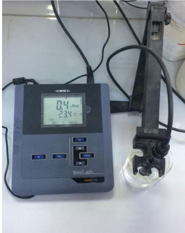
Figure B.1.9 Conductivity and Total Dissolve Solid TDS (InoLab Cond 7110 Supplied by WTW, Germany)
