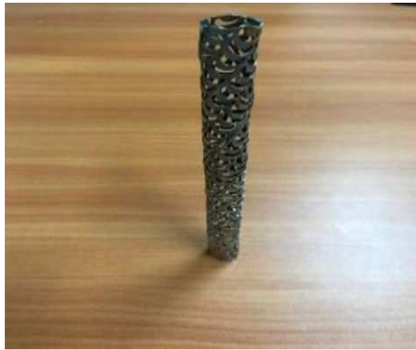
Figure 3.1 Represent the Outside Electrode form, it was Made from the (Silver and 4% Gold), Length = 14 cm, ID = 10.0 mm, OD = 10.4 mm.
