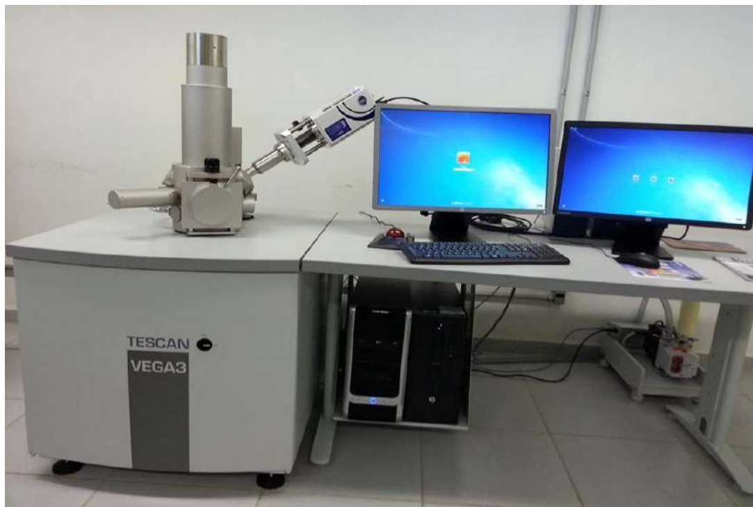
Figure B.1.3 SEM – EDXS (SEM Vega 3, Czech Republic, EDXS, Amertek Inc, Paoli, PA, USA)
