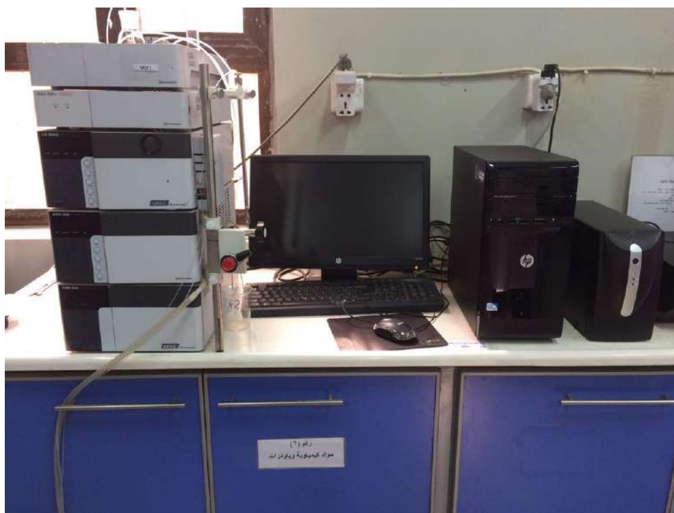
Figure B.1.6 High-Performance Liquid Chromatography (HPLC) (HPLC, model VQC1 supplied by SHIMADZU, Japan)
