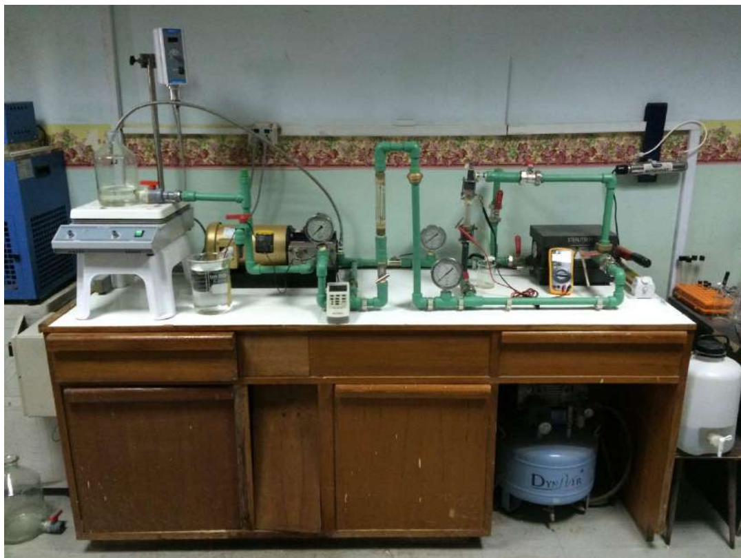
Figure 3.6 Bench Scale of Tubular Ceramic Titanium Dioxide NF Membrane and Flat Membrane Filtration Rig.
