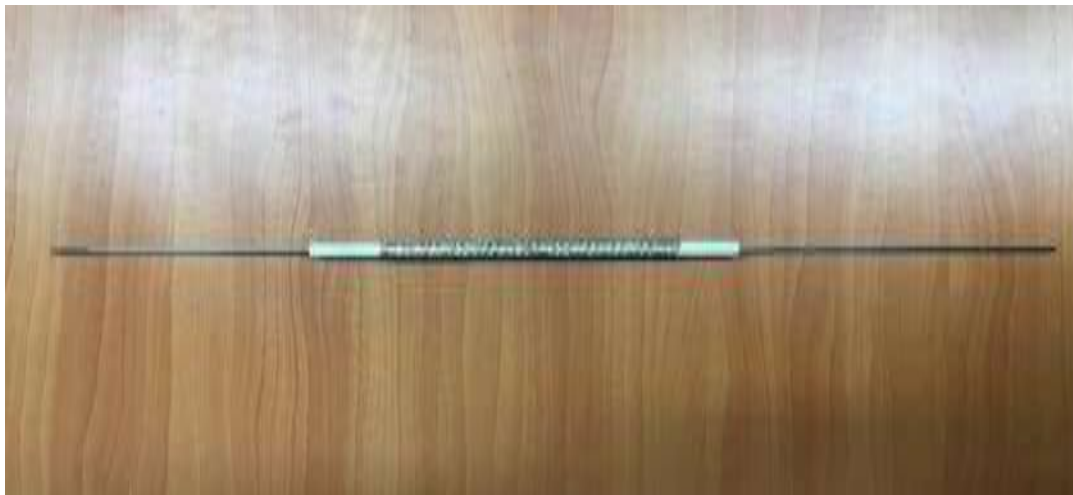
Figure 3.2 Represents the Inside Electrode form, it was Made from Composite (Silver and 4% Gold), Length = 50 cm, D = 4 mm which Passed in the Center Line of Ceramic Membrane and the Outside Electrode was Warped around the Outer Wall of Tubular Ceramic Membrane.
