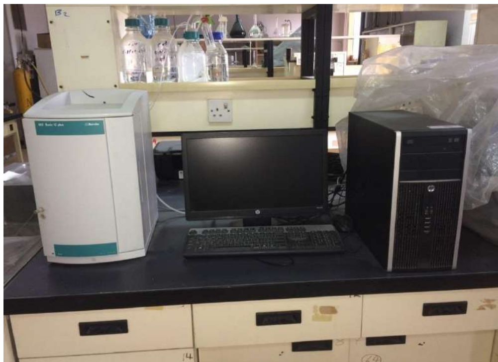
Figure B.1.4 Ion Chromatography (Metrohm Company, Model 883. Basic IC Plus, Swiss Origin)
