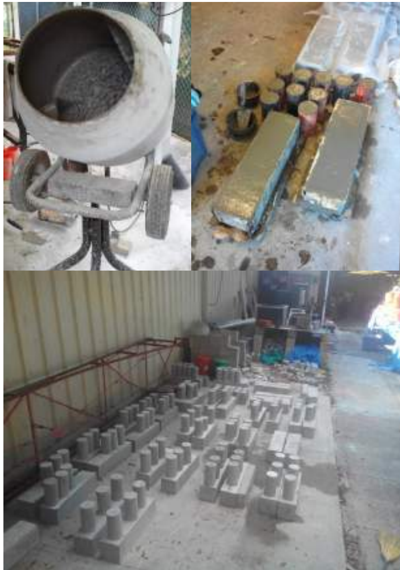
Figure 3-4: Specimens preparation of FRC and FRCC.
