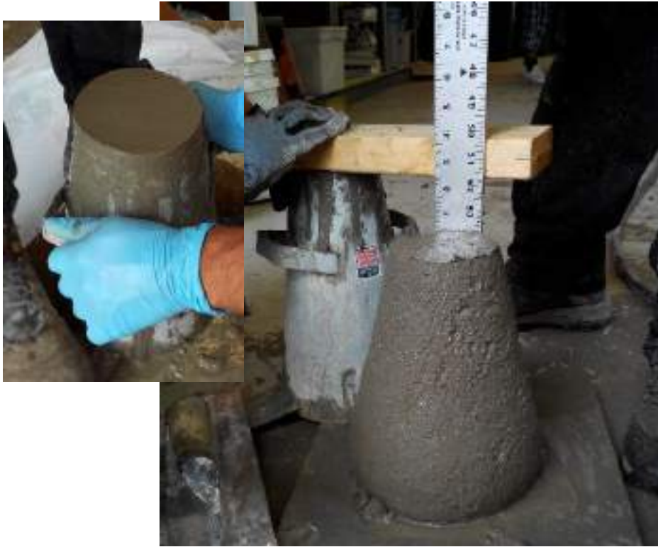
Figure 3-5: Slump cone test with the ASTM C143.
