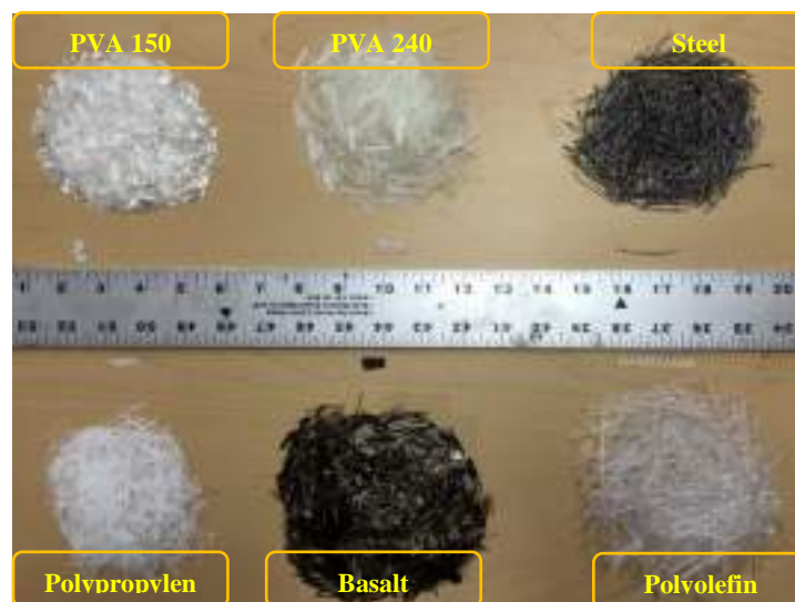
Figure 3-1: five types of fiber reinforced concrete.
