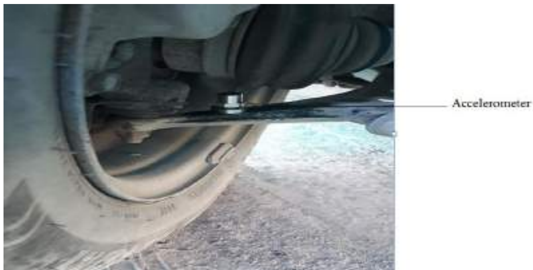
Figure(A-3) Placed the accelerometer on unsprung.
