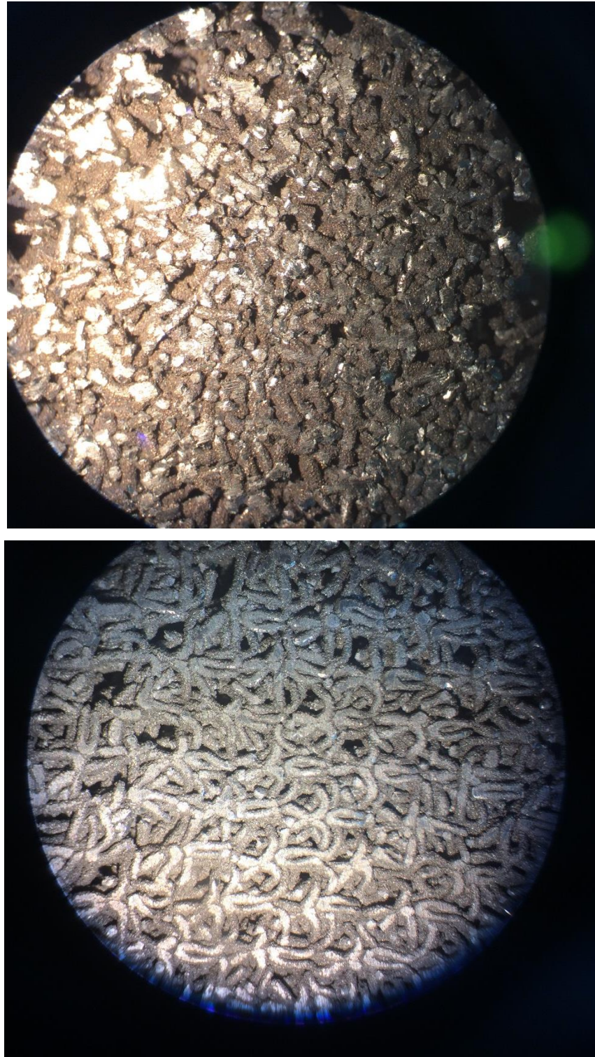
Figure 3 fracture morphology of the top layer ( lowest density) of graded lattice structures after compression tests, (Top) as-build , and (bottom) heat-treated conditions.
