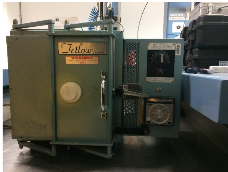
Figure 5.8 electric furnace with air atmosphere
