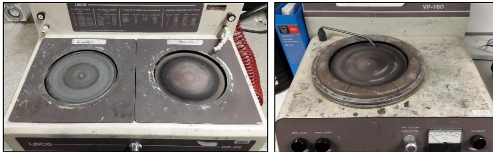
Figure 5.6 (A) Polishing machine with 3 & 6 \mu\text{m} , (B) Polishing machine with 1 \mu\text{m}
