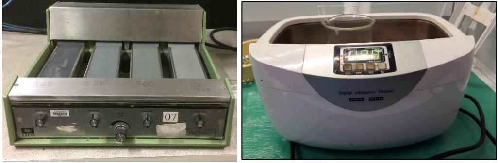
Figure 5.5 (A) Grinding machine (B) Ultrasonic device
