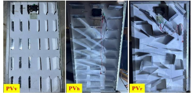
Figure 3. Modified PV panels with various fin orientations
