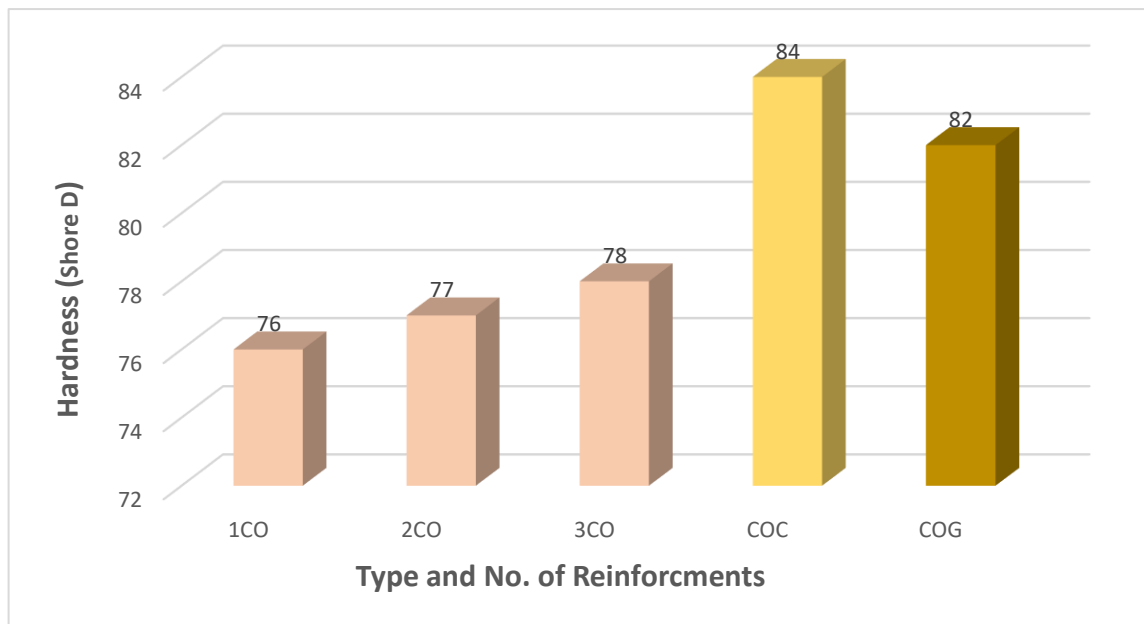
Figure (6.28): Hardness (Shore-D) of Laminated Composite Materials and Woven Cotton Fibers layers for prosthetic sockets.
