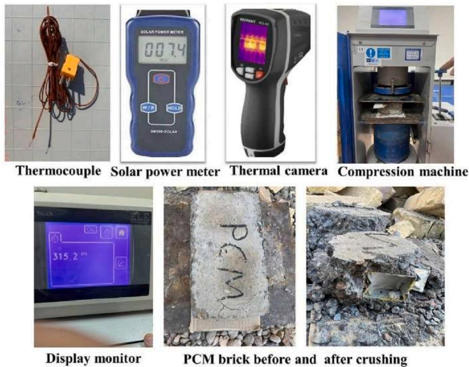
Fig. 4. Photos of thermal measurement devices and mechanical test machine.
