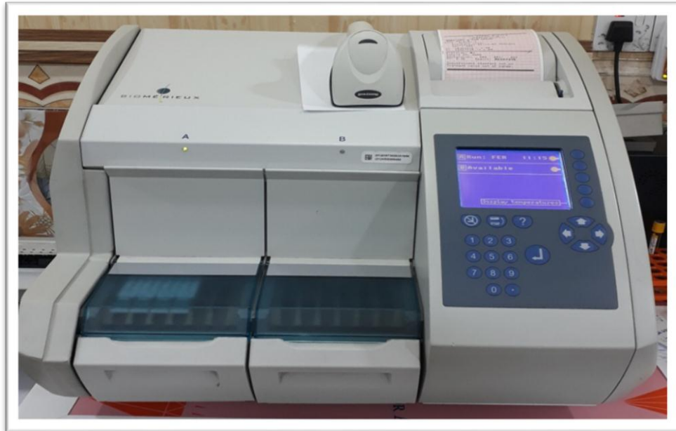
Figure (3-4): Minividas device works to read ferritin in the serum of patients with Covid-19
