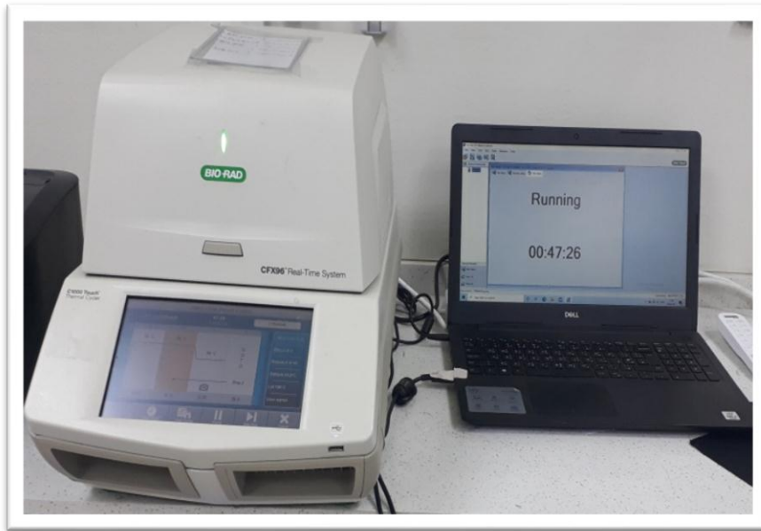
Figure (3-1): Thermal cycler PCR device determines the result of a positive or negative nasal swab for Covid-19 patients.
