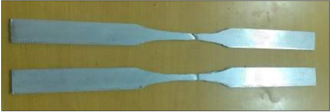
Figure (3.7) Aluminum alloy tensile coupons after test
