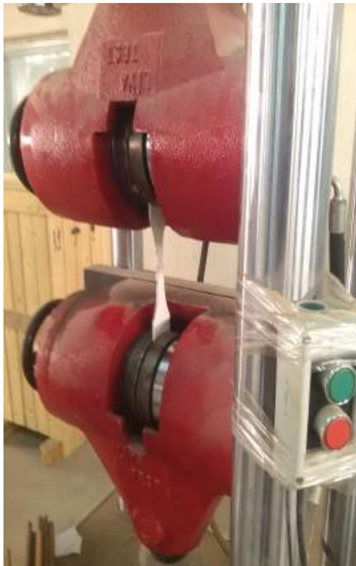
Figure (3.6) Test arrangement for aluminum alloy tensile coupons
