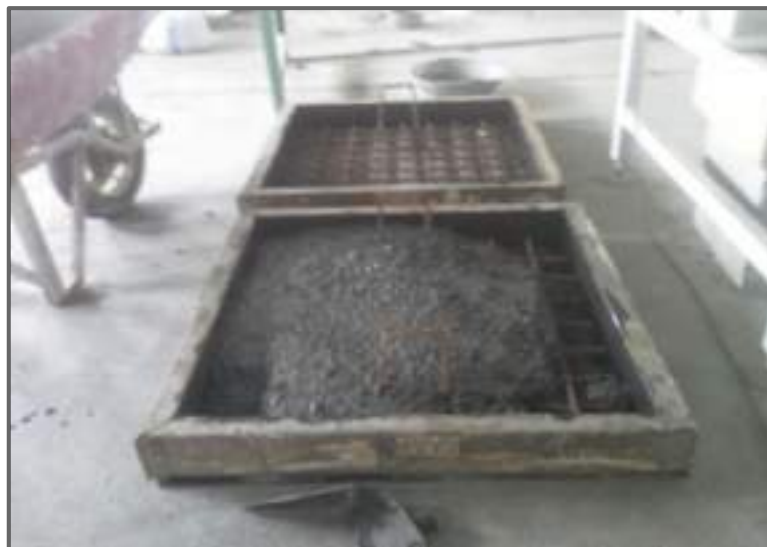
Figure (3.18) the molds used in the casting process
