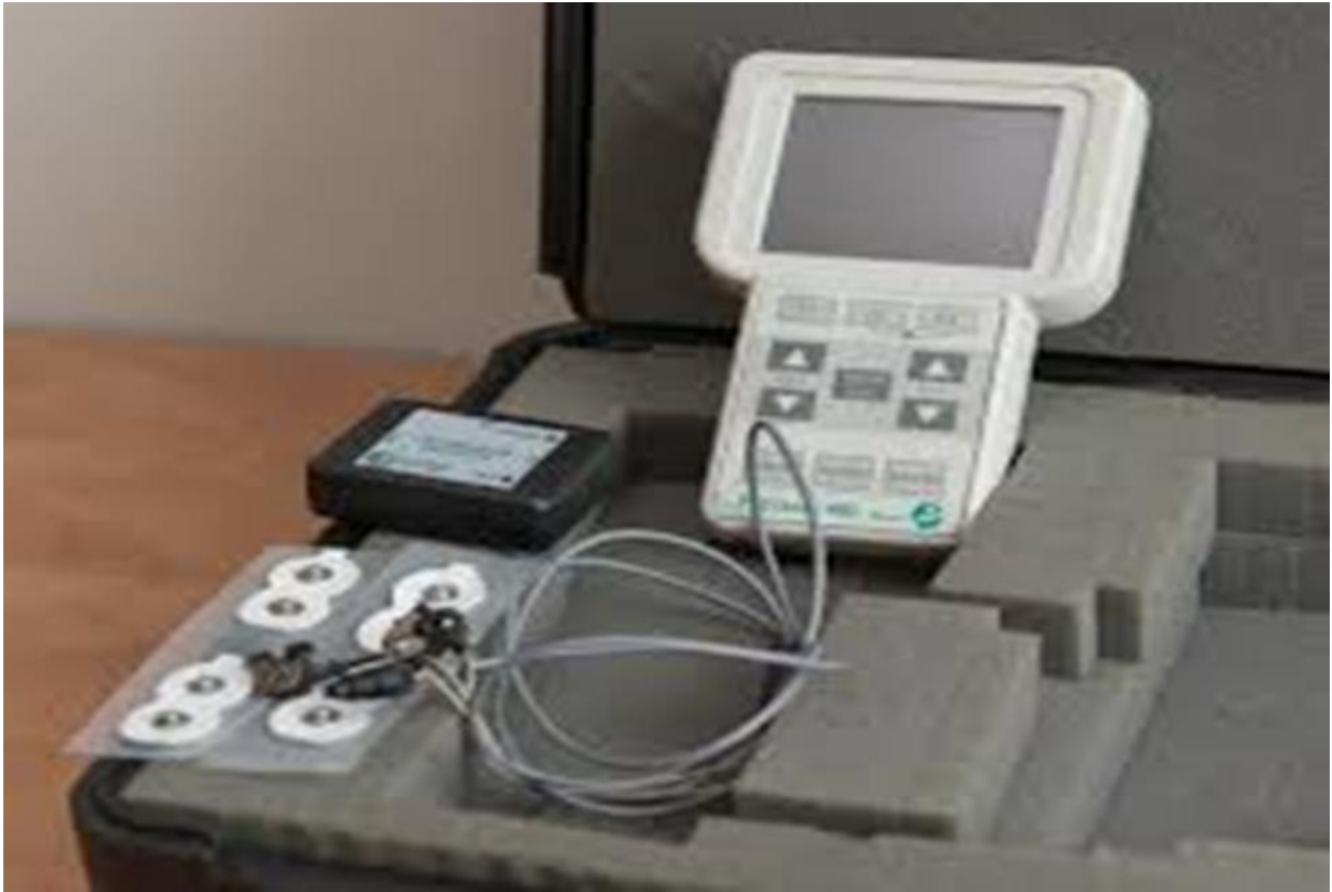
Figure (4-4) the cutting-edge electromyography (EMG) Myotrace 400 device.
