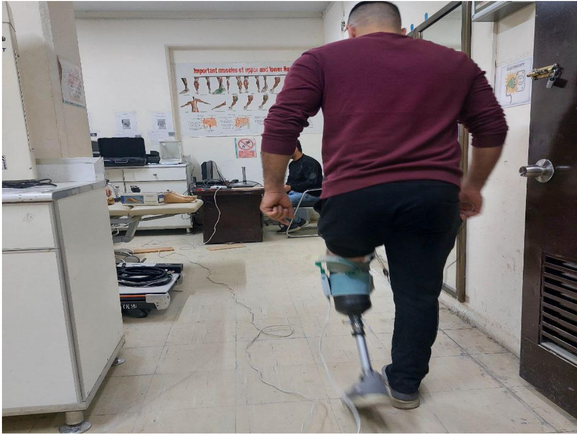
Figure (4-9) Measurement of socket pressure distribution.
