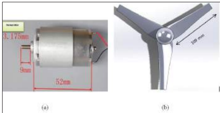
Figure 4.19 Micro-wind turbines: (a) Micro Generator (b) Three blades of airfoil NACA4415 and Nacelle
