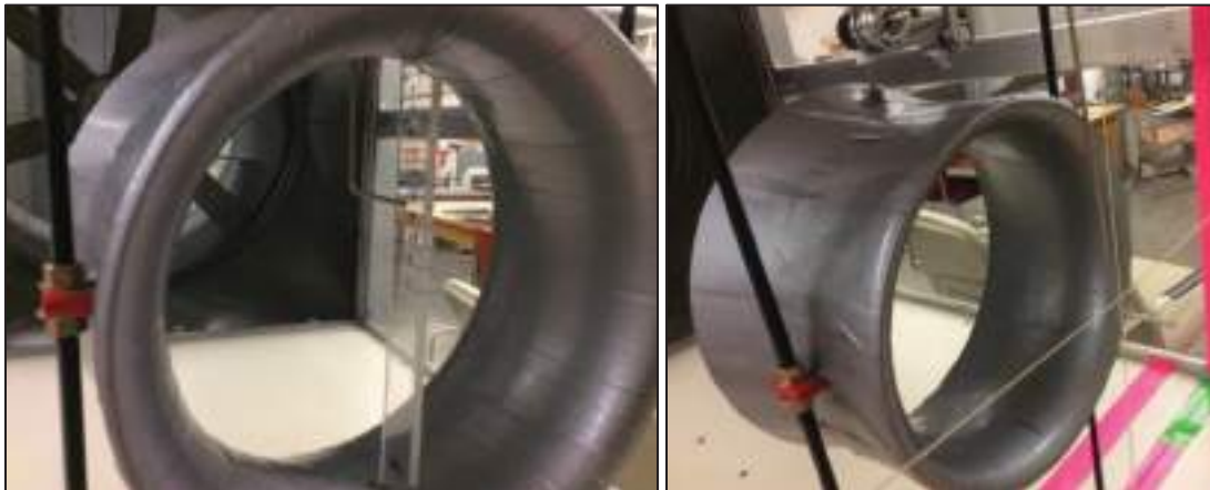
Figure 4.18 Pitot static tubes placed inside and outside the shroud
