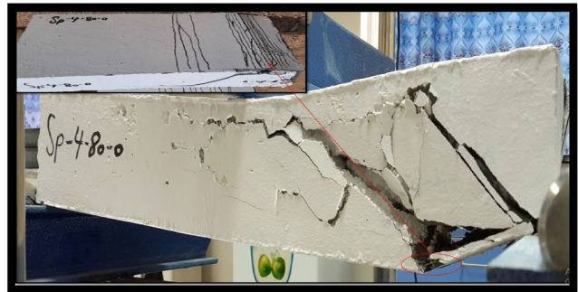
(b) Mode of failure for Sc-4-80-0.
