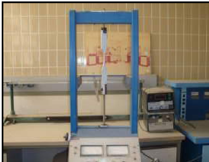
Plate (3-4) Test arrangement for aluminum alloy tensile coupons
