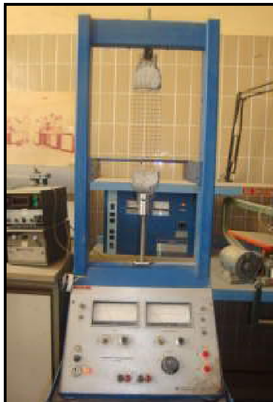
Plate (3-8) Test arrangement for wire mesh tensile coupons
