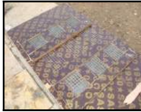
Plate (3-5) Fabrication details of wire mesh tensile coupons specimens
