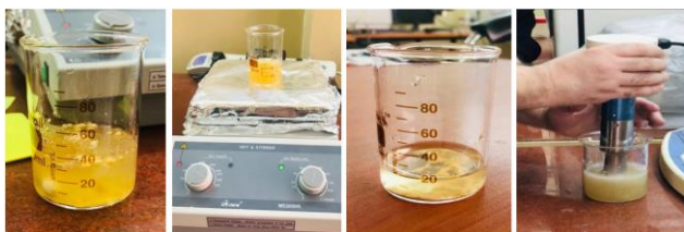
Figure 1. The steps of preparation of the biocomposite coating
