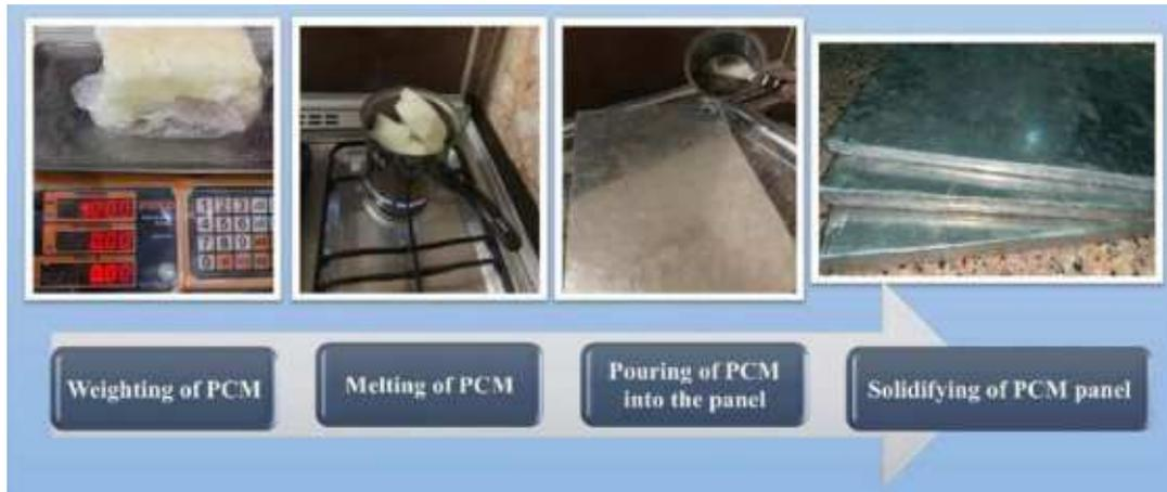
Fig. 3.10. Preparation procedure of PCM panels
