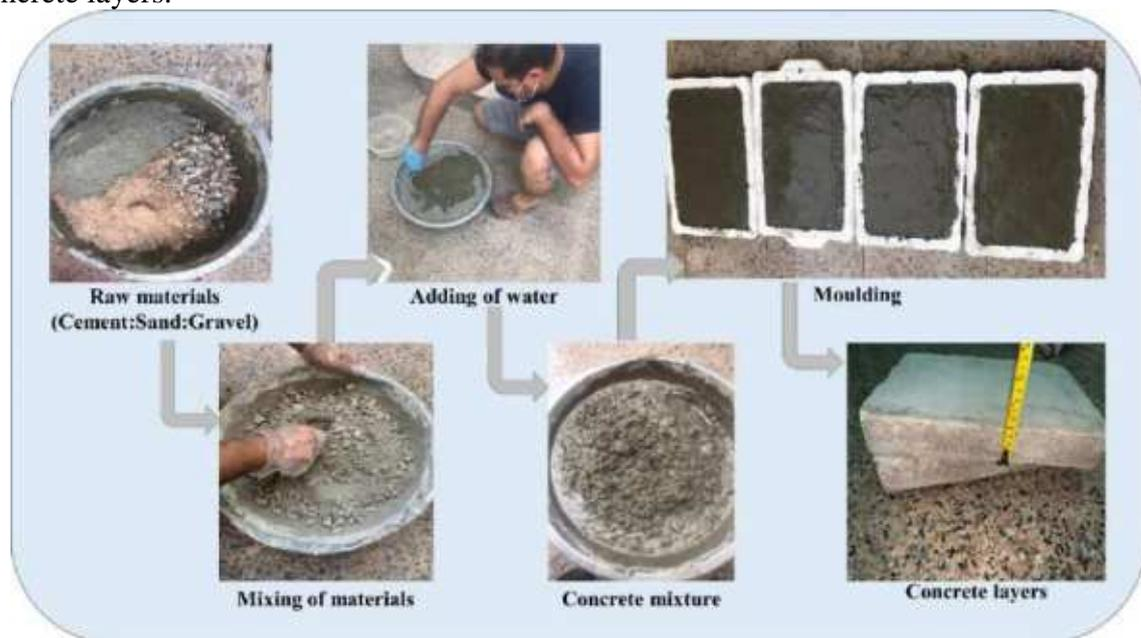
Fig. 3.5. Fabrication procedure of concrete layers
