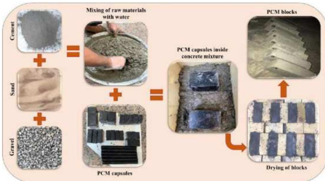
Fig. 3.12. Fabrication procedure of PCM concrete bricks
