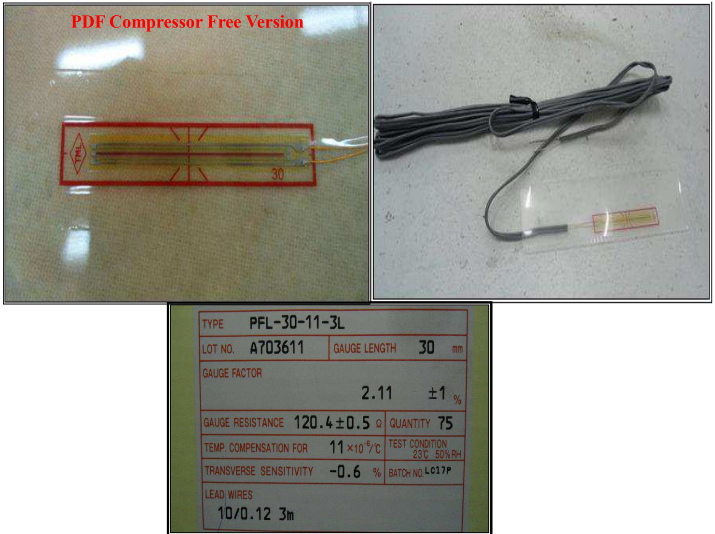
Plate(3-8): Electrical strain gauges used for measuring concrete strain
