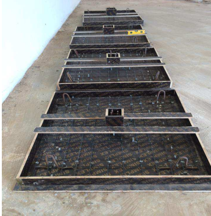
Plate(3-5): Molds used to cast the specimens
