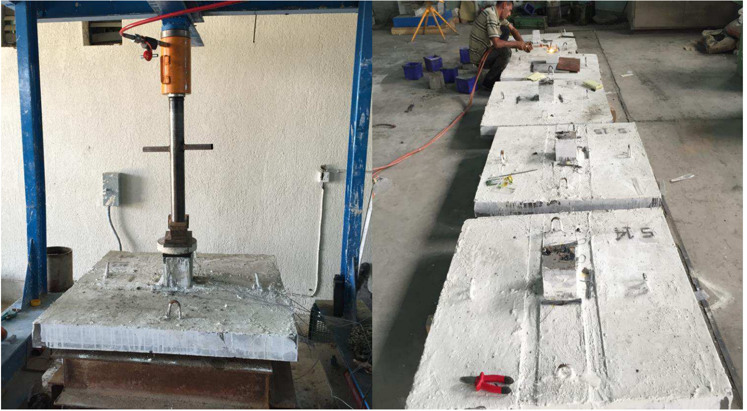
Plate (3-9): Testing mechanism and treatment of slab specimens before testing
