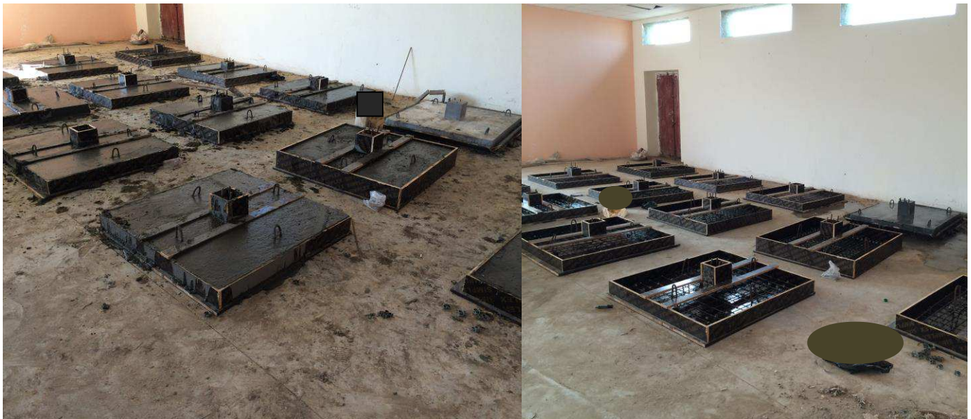
Plate(3-6): Casting of RPC slabs
