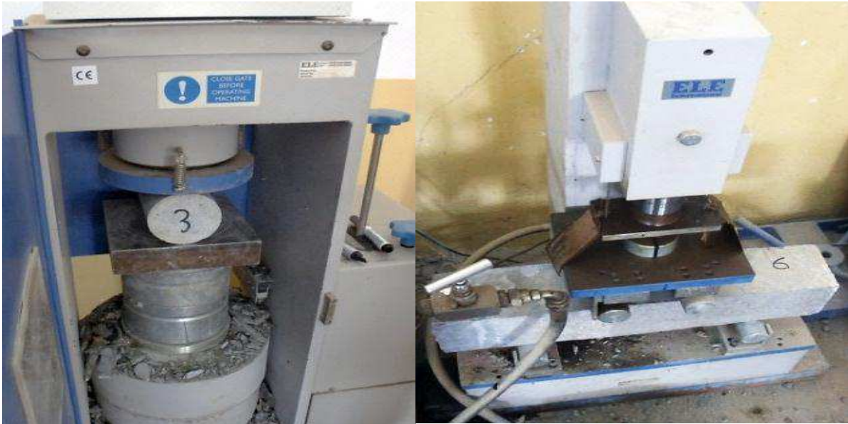
Plate (3-4): Test of mechanical properties of RPC
