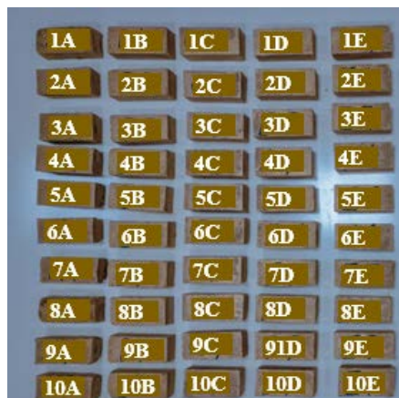
Fig. 4: Specimens of fired clay brick for all mixes of stone powder.
