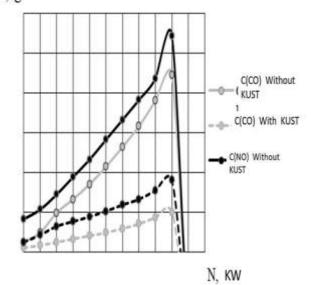
Figure 5. Dependence of CO and NOx concentrations in the exhaust gas on engine power
