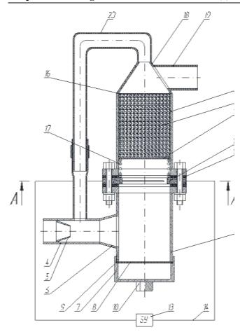
Figure 1 .General view of the diesel KUST 1 - catalyst bed; 2 - the upper part of the body; 3 the lower part of the body; 4 - pipe; 5 - ejector; 6 diffuser; 7 - sump filter; 8 - metal mesh; 9 - gasket; 10 - a nut; 11 - electric spiral; 12 - sealing gaskets; 13 - control unit; 14 - electrical wires; 15 - entrance
