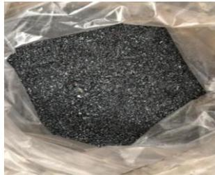
FIGURE 2. Iron filings particles.
