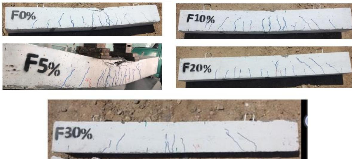
**FIGURE 16.** Cracks pattern for beams specimens containing iron filing as a sand replacement.
