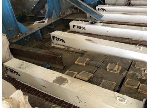
**FIGURE 6.** Reinforced concrete beam specimens for all iron filing/sand percentages
