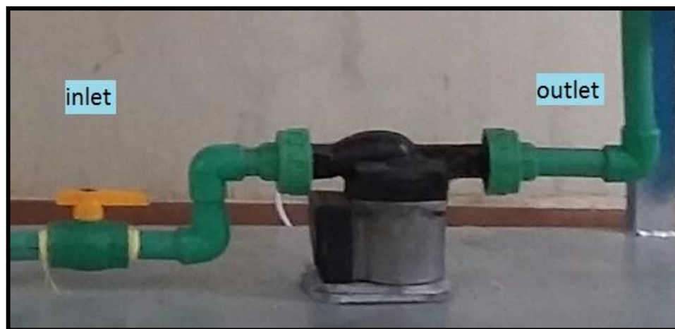
Fig.4.4 Thermal Circulating Pump
