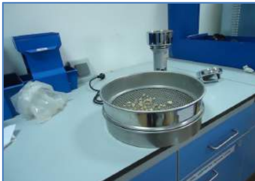
Fig. 3.5 Sieving the sample
