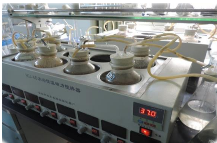
Figure 3-1 Batch reactors fitted in water path
