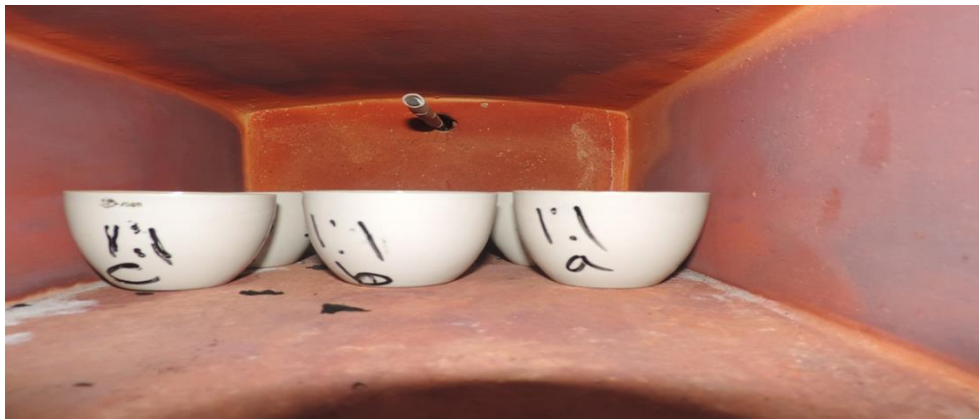
Figure 3-7 Measure the volatile solids by placing the dried samples in the combustion furnace at a temperature of 550 ° C for 2 hour
