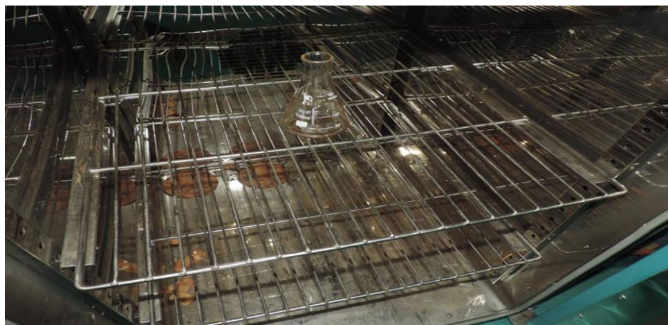
Figure 3-15 Place the flask inside a drying oven for 1 hour and 100 ° C
