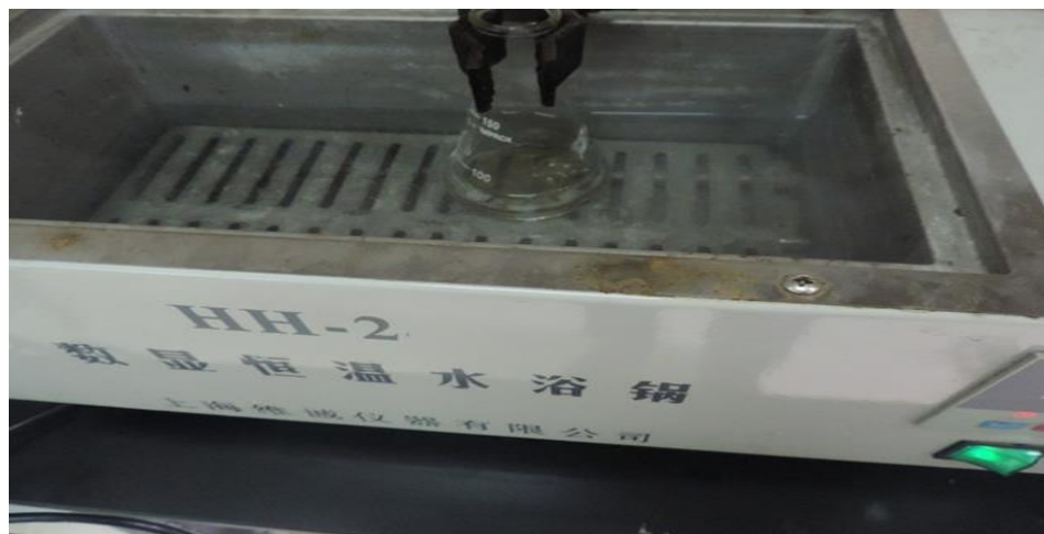
Figure 3-14 Place the flask inside a water bath for 1 hour and 80 ° C
