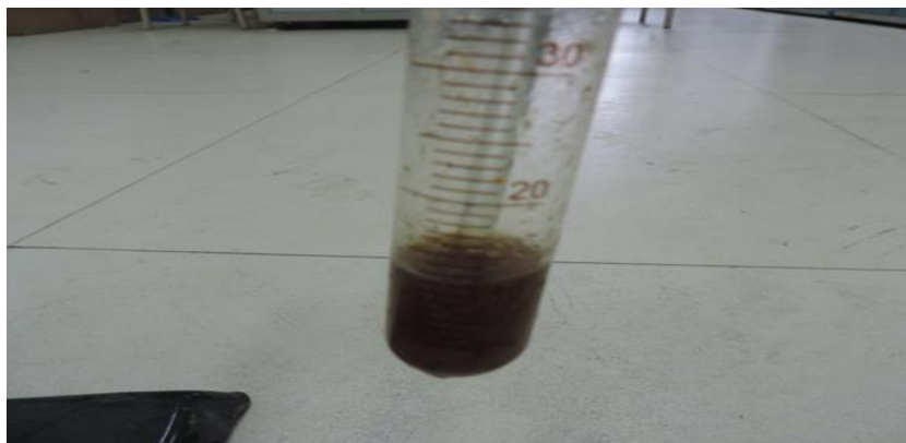
Figure 3-10 Dissolve the food after adding hydrochloric acid
