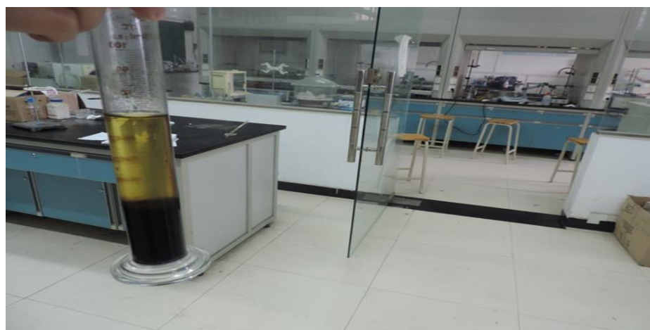
Figure 3-11 After the addition of hydroxide acid, the tube was placed water bath at 75.6 c for 40 minutes
