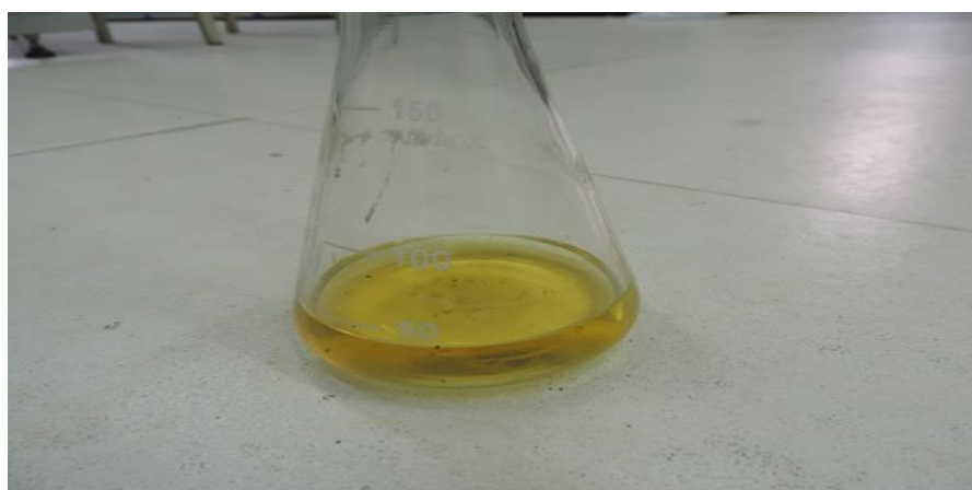
Figure 3-13 Transfer the oil from the tube to the flask by pipette
