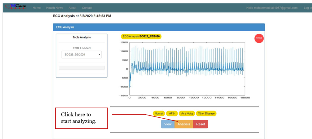
Figure 5.40 View ECG Signal by the ECG Analysis Page
