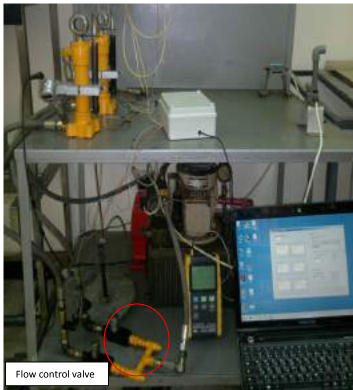
Fig. (4-11): The experimental apparatus to FCV (no load no linkage.) with the schematic diagram.
