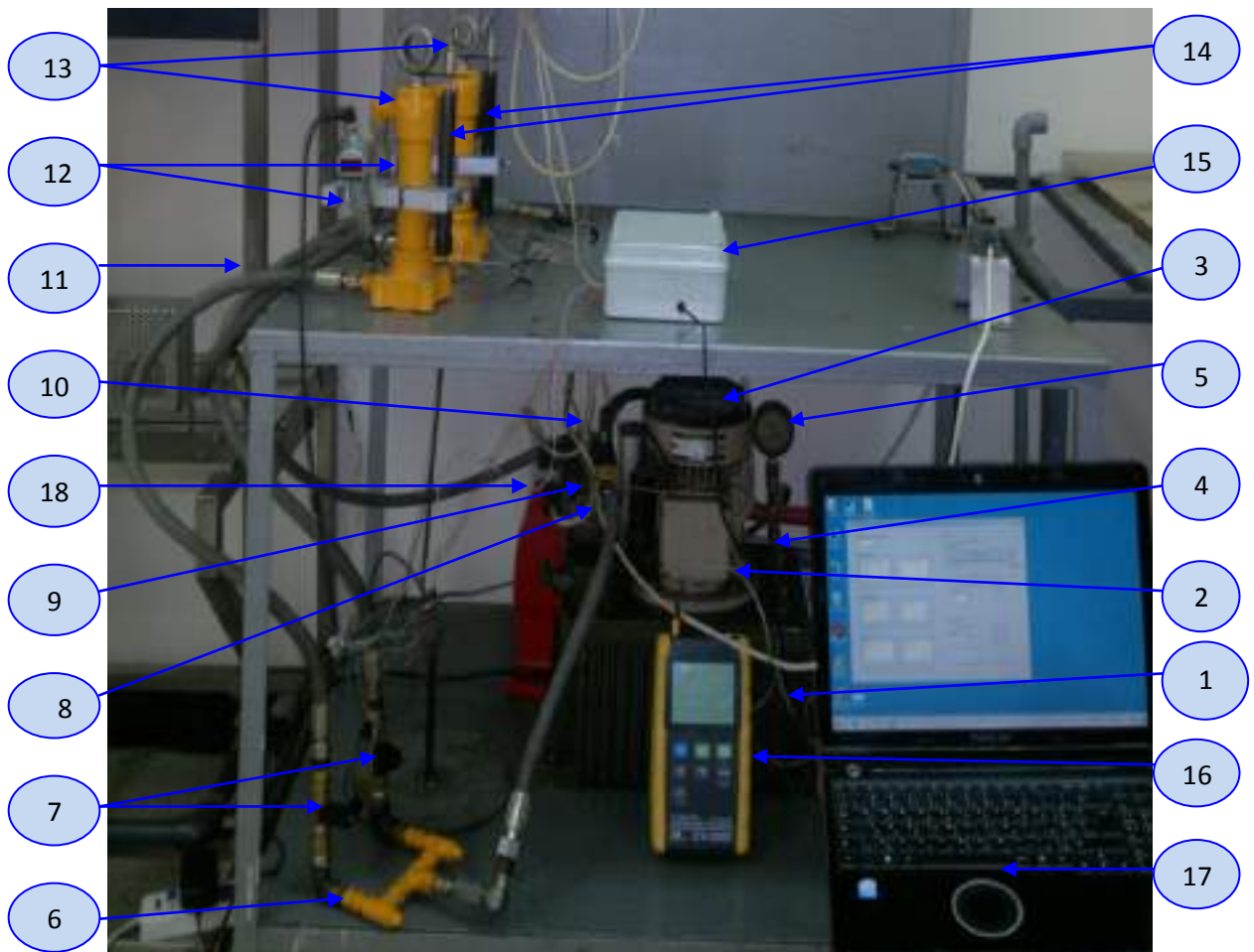
Fig. (4-5) The experimental apparatus for Tee connection (no load no linkage).
