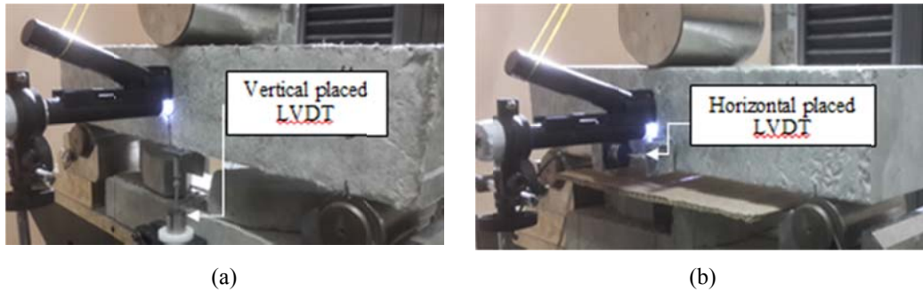
Figure 2 Linear Variable Displacement Transducer (LVDT) located (a) at the bottom of the center the specimens (b) at the side of the specimens
