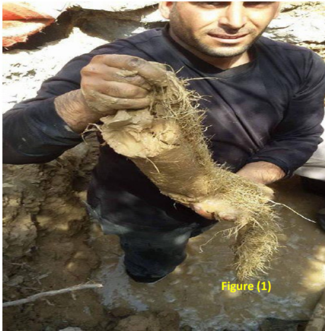
Fig. 1 : shows The roots are pierced in the water pipe in Al-Ressala Sector
