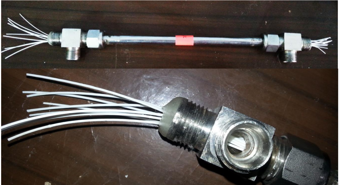
Figure 3.5: Picture for Membrane Module.
