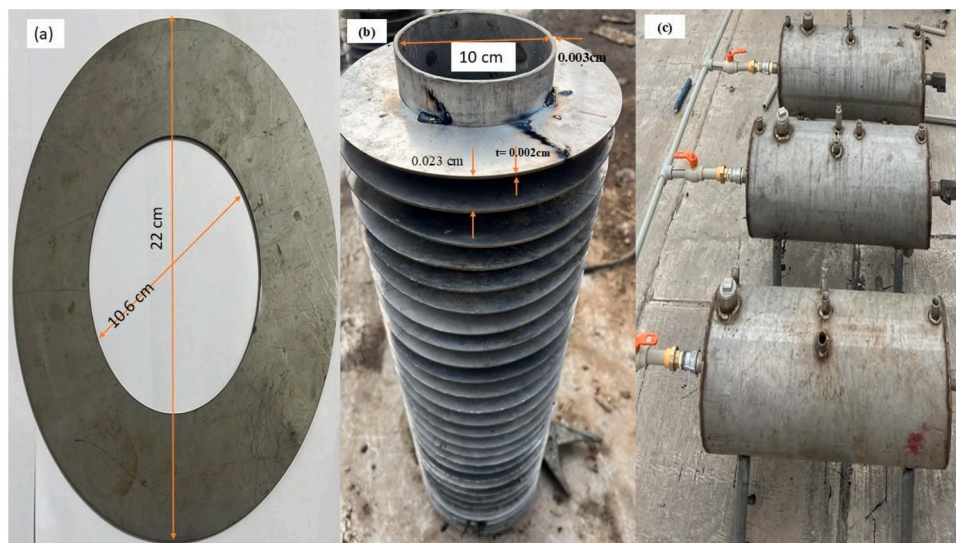
Fig. 1. (a) ring fins, (b) ring fins welded on the inner tube, (c) experimental tanks.
