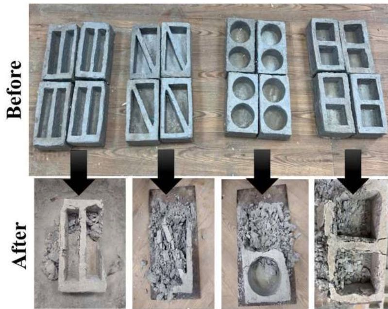
Fig. 14. Test bricks before and after the compressive strength test.
