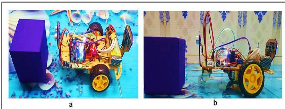
Fig. (4.22): Obstacle detection at forward direction: (a) the result recorded from the top, (b) the result recorded from one side.
