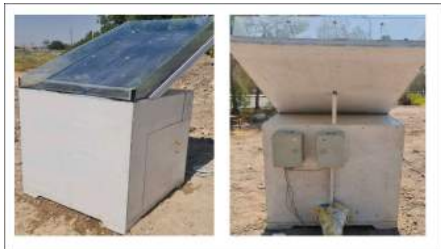
Fig. 6. Photo of the solar chimney with room experimental system.
