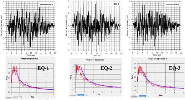
Fig.(5): Acceleration-Time Histories of Artificial Earthquakes Its Spectra
