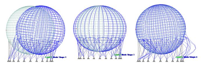
Fig.(2): Mode Shapes of LPG spherical Tank for First Four Modes
