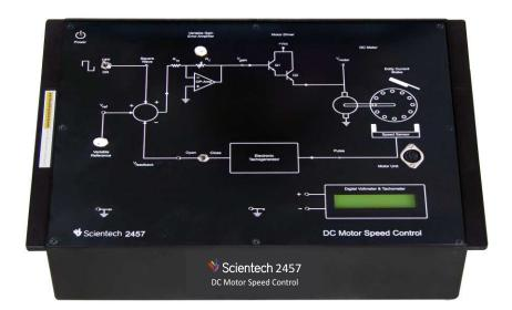
**Scientech 2457 DC Motor Speed Control** is built around a compact permanent magnet DC Motor. The system can readily be configured to control speed of DC Motor using Pulse Width Modulation technique. Motor load can be varied by using built in eddy current brake. Facilities are available to directly measure the principal performance features of the speed control system, viz, steady state error and load disturbance rejection, as a function of the forward path gain.
