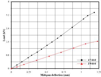
\*\* Flexural ductility is the ratio of deflection at ultimate load to deflection at the end of linear region.
