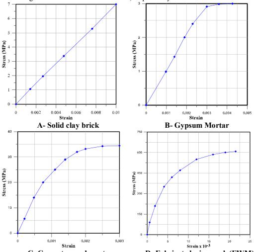
C- Cement – sand mortar D- Fabricated wire mesh (FWM) Figure (1) Stress –strain relationships of used materials in brickwork arches Fabrication
