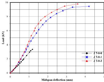
Figure (6) Reinforced finishing layer (Ferrocement) effect upon strength and variation of mid-span deflection with applied load
