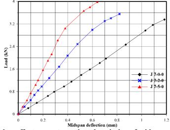
Figure (5) Camber effect upon strength and variation of mid-span deflection with applied load for jack arch specimens
