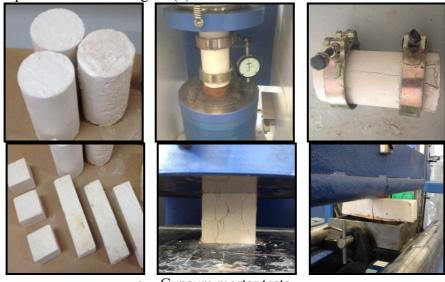
a- Gypsum mortar tests
