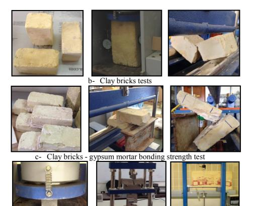
d- Ferrocement components tests (cement mortar an fabricated wire mesh) Plate (3) Material properties tests
