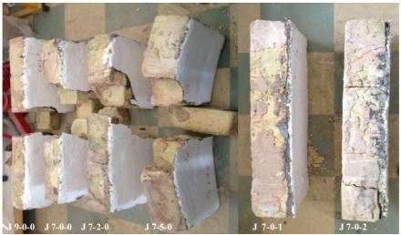
Plate (6) Failure modes
