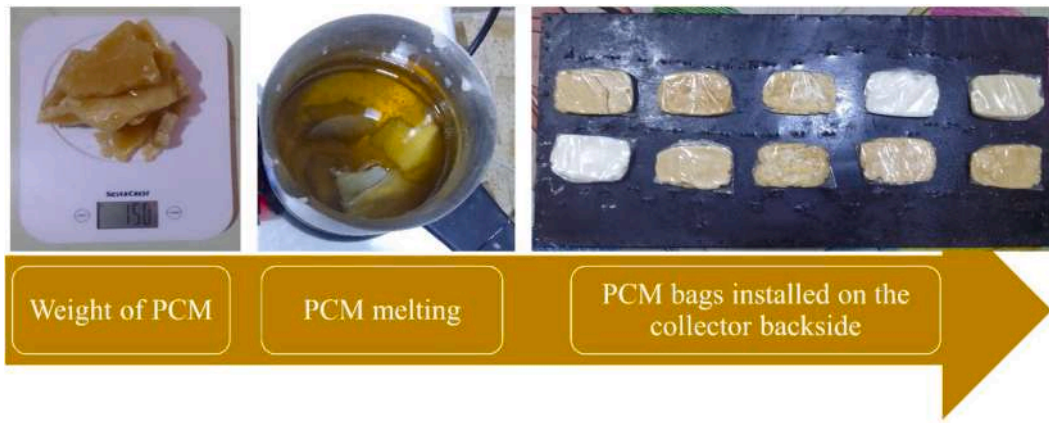
Fig. 3. Preparation procedure of PCM thermal bags.
