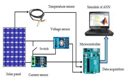
Figure 4. Block diagram of the proposed method.
