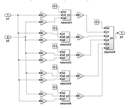
Figure 6. The Simulink model of the trained neural network (NN).
