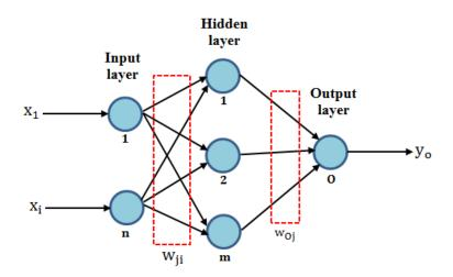
Figure 3. Three-layer neural network.
