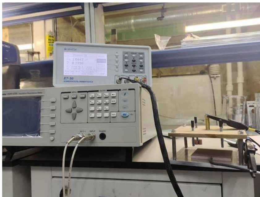
Figure 3.17. Connecting the E7-30 to the measuring cell.
