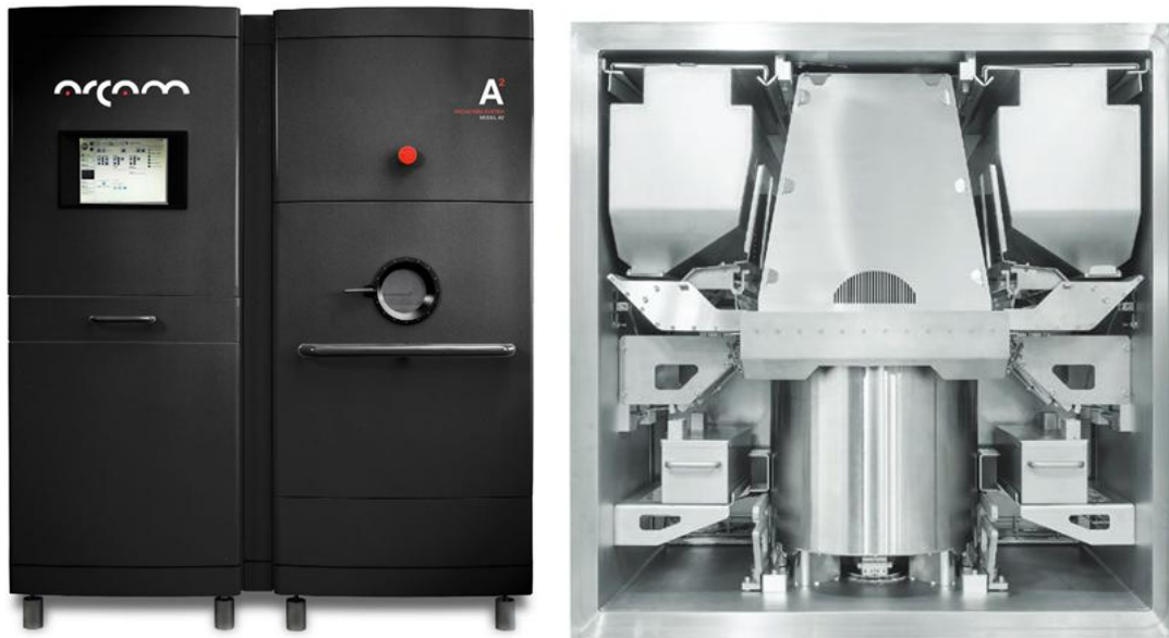
Figure 2.4. Arcam A2 electron beam melting unit
