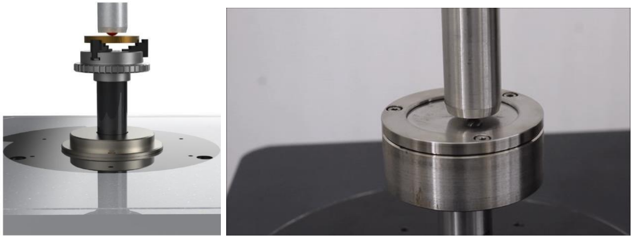
Fig.2.16. DUCOM POD-4.0 friction unit
