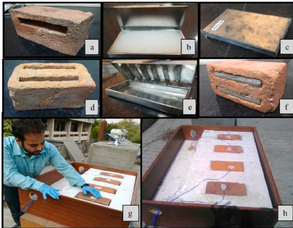
Fig. 21. Fabricating steps of PCM-incorporated bricks; (a) Single-slot brick, (b) Encapsulation container, (c) Macroencapsulated PCM, (d) Double-slot brick, (e) Encapsulation container with fins, (f) PCM-incorporated brick with twin slots, (g) Installation of bricks and (h) Final setup [58].
