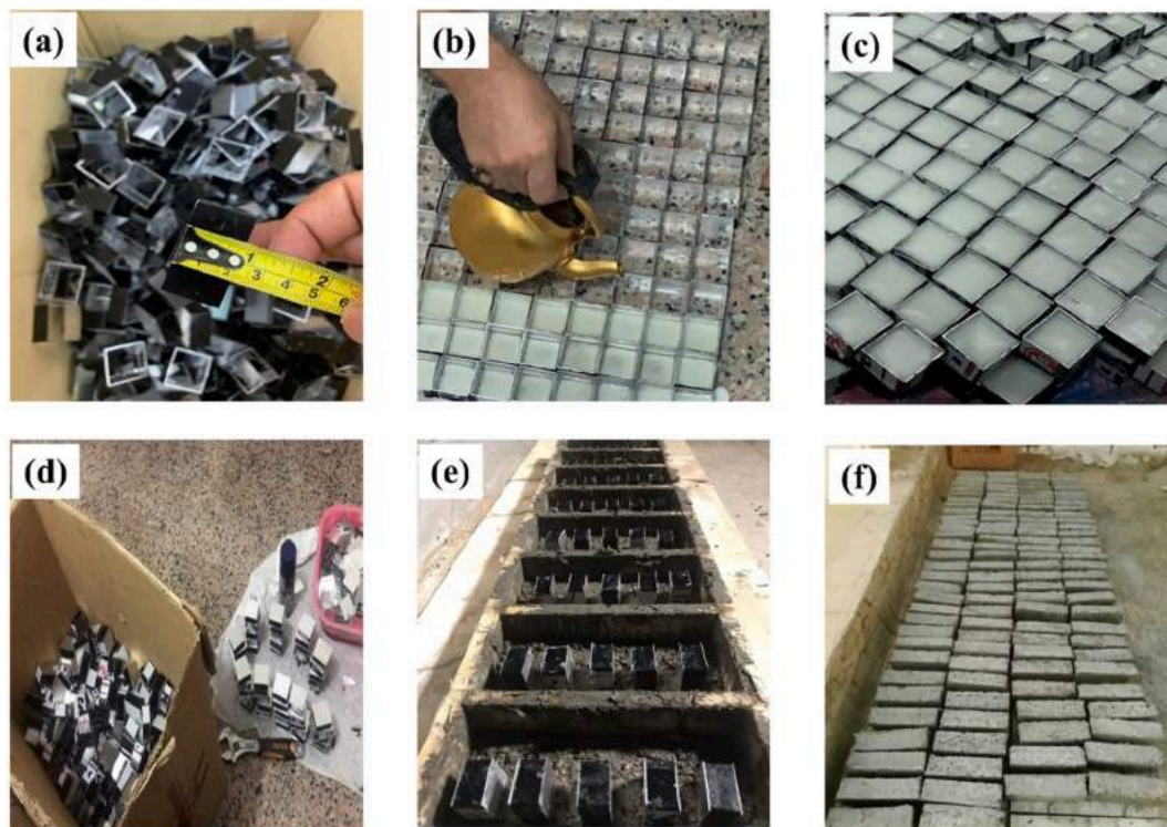
Fig. 3. Preparation of PCM bricks: (a) aluminium capsules; (b) pouring of liquid PCM; (c) solidified PCM capsules; (d) capping of PCM capsules; (e) PCM capsules inside concrete during preparation; (f) dried PCM bricks.
