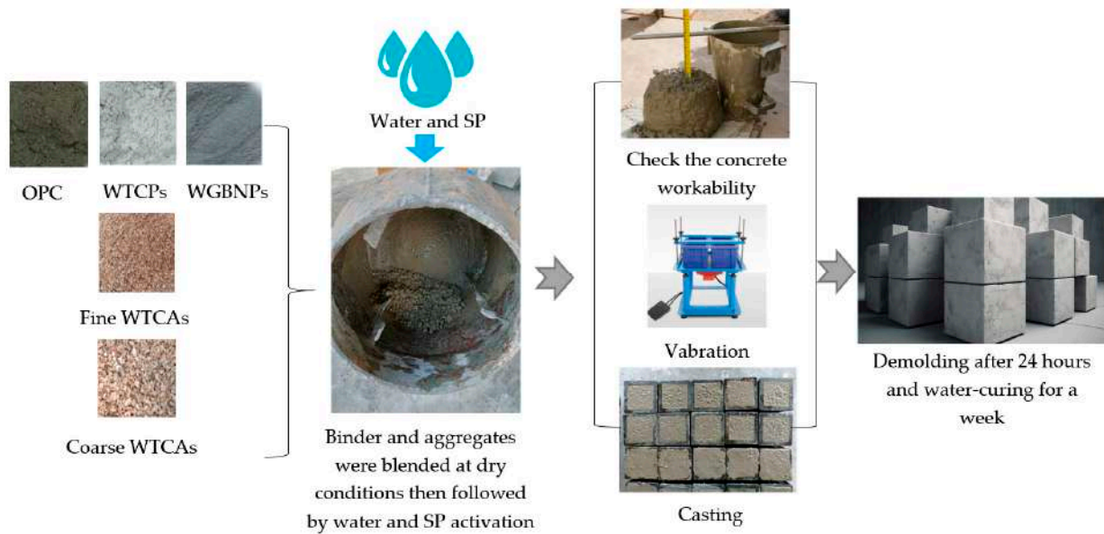
Figure 2. Proposed concrete specimens' preparation procedure.
